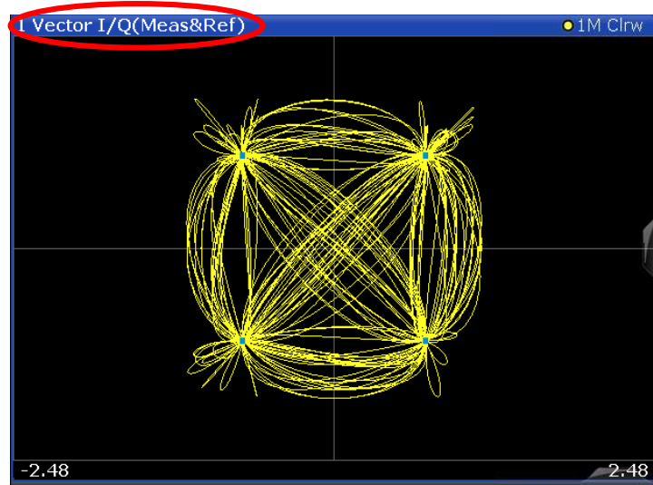
Vector Diagram (IQ location at symbol clock and during transitions)
