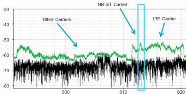
A more pervasive issue is in-band interference. Receivers can be de-sensitized by any RF signal that reaches their first mixer. Since the low cost NB-IoT receivers are not likely to have a pre-filter, a generally high noise floor on the downlink band can cause a loss of sensitivity of the NB-IoT device receiver. That can be a real issue when the device is in a location with high path loss.
