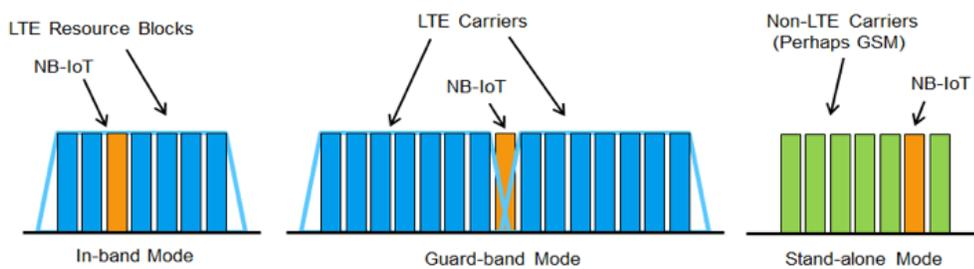
NB-IoT supports three different operational modes: In-band operation, guard-band operation, and stand-alone operation.
