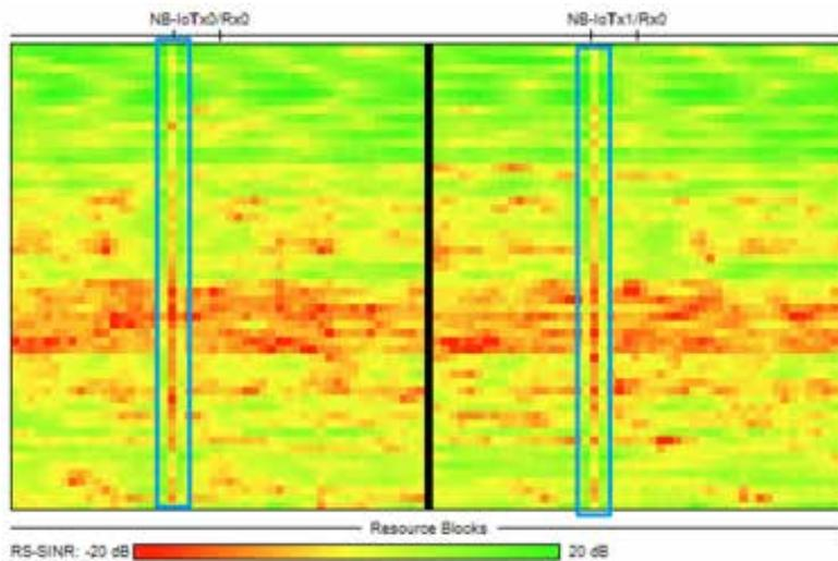
Figure 5: RS-SINR visualization of LTE with in-band NB-IoT.
