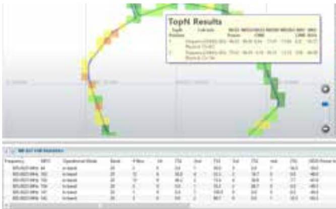
Figure 7: Mapped display of detected problem spots along the drive test route.
