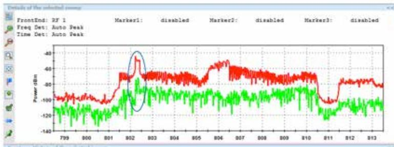
Figure 6: RF Power Scan view of NB-IoT Power Boost within an LTE signal.
