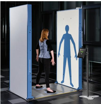
The R&S(QPS) allows a more natural scanning pose and automatically alerts the system operator of improper positioning.
