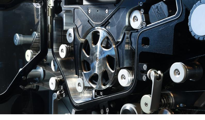
The Hamburg location has been equipped with a storage area and a 4K film scanner – the dft Scanity HDR with wetgate technology for 16 mm and 35 mm films. In the wetgate method, the film passes through a tray of perchloroethylene. With a refractive index very close to that of the film, this chemical compensates for scratches and cracks in the material during scanning.
