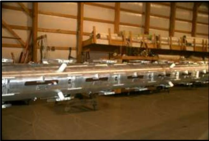
**Figure 6: Slot antenna.**
