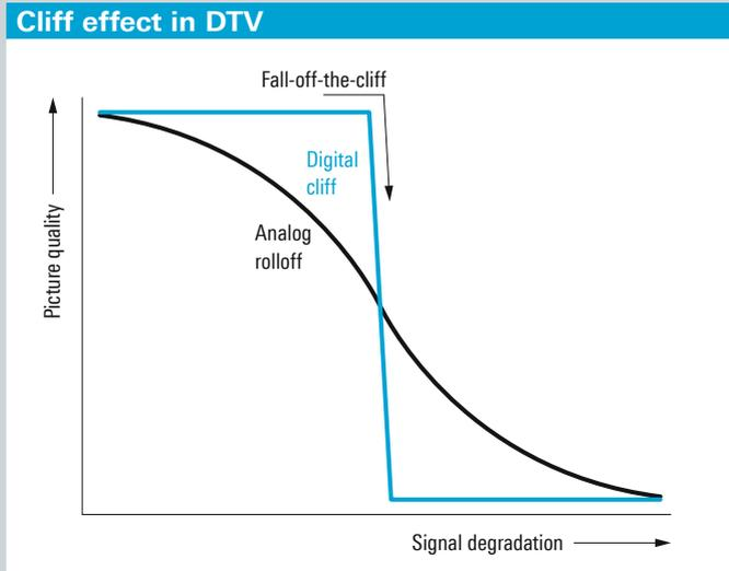
If these minimum MER values are not reached, a cliff or brickwall effect can occur. In such cases, it is suddenly no longer possible to receive the TV or audio broadcasting signal after minimal degradation in signal quality.
