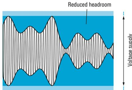
Adjusted voltage supply – higher efficiency
