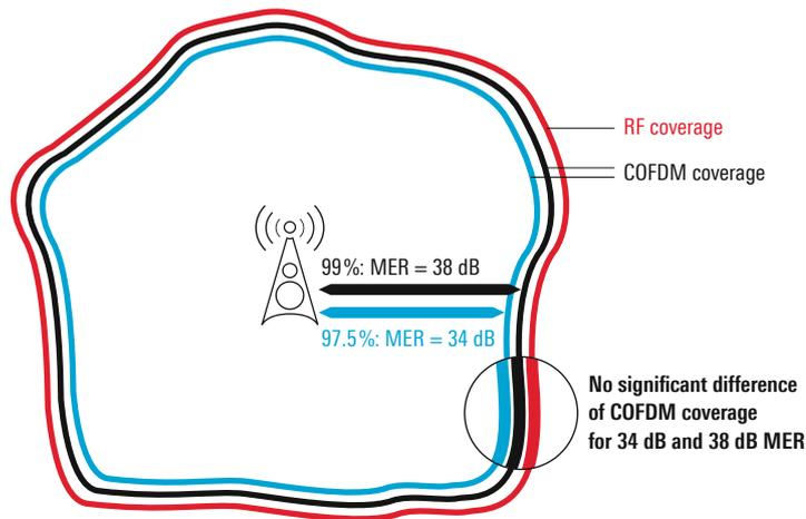
38 dB results in a difference of just 1.5 percentage points referenced to the equivalent reduction of the relevant transmit power. In this example, increasing the MER would barely expand the covered area at all.
