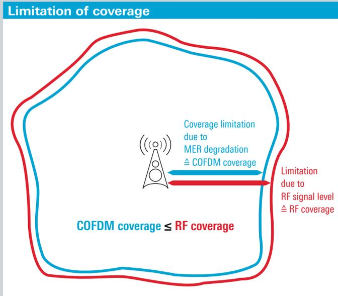
If, for example, the transmitter provides a signal with an MER of 16 dB above the fall-off level, this has an influence of about  $-0.1$  dB on the receiver MER. With regard to RF coverage, this influence corresponds to a reduction in transmit power to approx. 97.5%. If the signal at the transmitter has an MER of 20 dB above the fall-off level, the influence on the receiver MER is  $-0.04$  dB,
