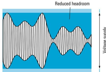
Adjusted voltage supply – higher efficiency
