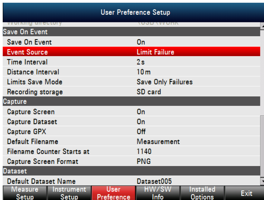
Fig. 6 Save On Event for limit failure in the User Preference Setup menu.
