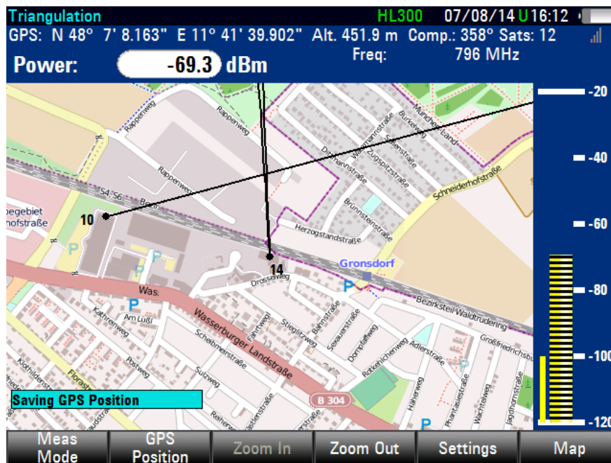
Fig. 20 Message in map triangulation display. Saving a GPS position with bearing using R&S®HL300 switch.
