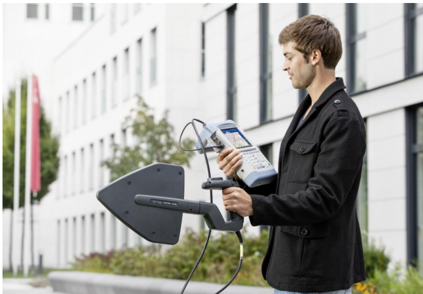
Fig. 13 Locating interference source with the FSH and the R&S®HL300 directional antenna.
