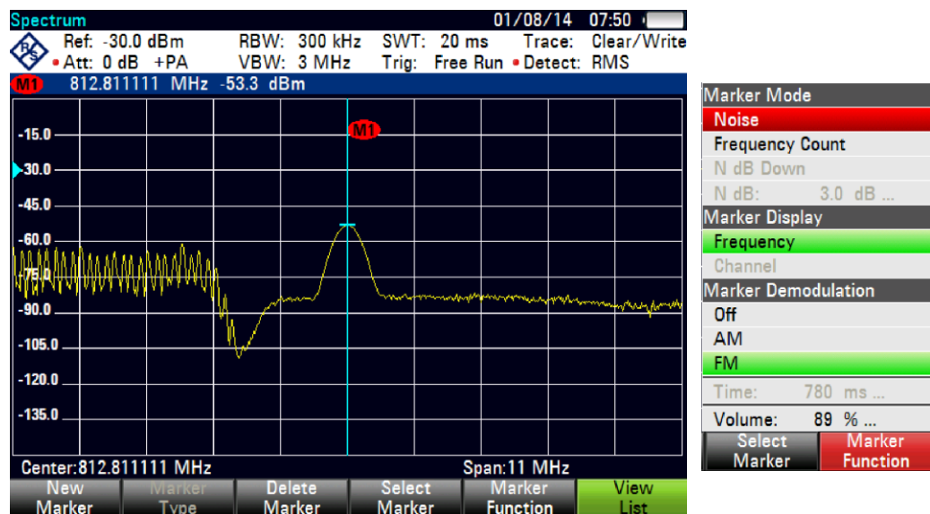
Fig. 37 FM modulated wireless microphone operating in the 800 MHz band. Marker Function menu.
