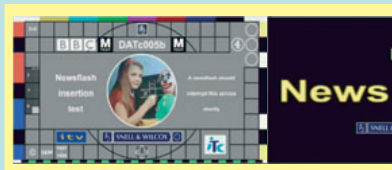
FIG 4 Sequence with temporarily inserted elementary stream.
