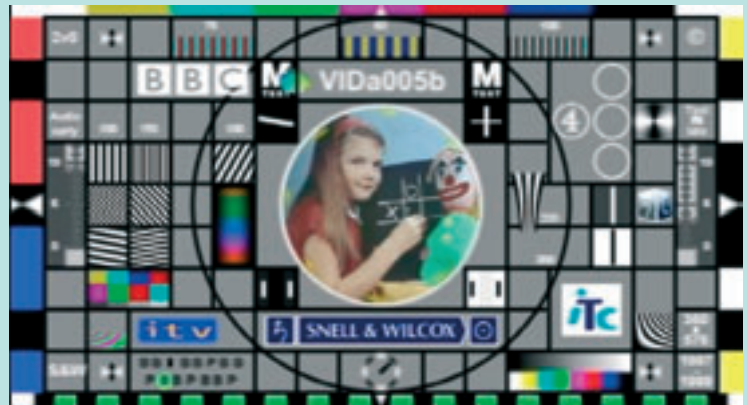
FIG 2 Test pattern with reduced horizontal resolution (360 pixels).
