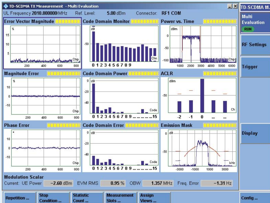
FIG 4 Based on identical sample sets, the multi-evaluation measurement allows the parallel evaluation of the measured signal. The measurement determines the error vector magnitude (EVM), magnitude error, phase error, frequency error, I/Q origin offset, I/Q imbalance, adjacent channel leakage ratio, spectrum emission mask, occupied bandwidth, code domain power and peak code domain error power.
