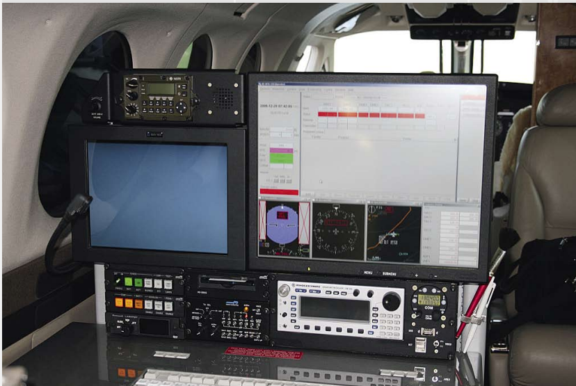
FIG 5 Part of the flight inspection system in the interior of the flight inspection aircraft.
