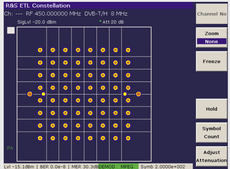
FIG 3 Constellation diagram of a DVB-T/-H signal (additional C/N = 30 dB).
