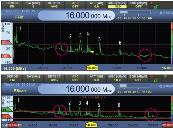
Fig. 2 Top: Fixed frequency mode (FFM) within the realtime bandwidth of 32 MHz at a resolution of 10 kHz. Bottom: Panorama scan (PS) mode with resolution refined to just 1 kHz captures more emissions (highlighted in red).
