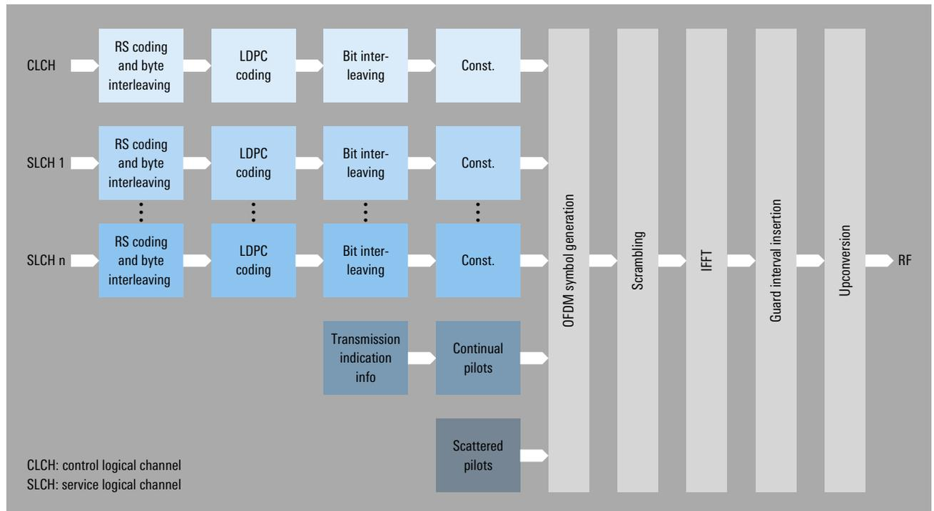
FIG 3 CMMB physical layer with logical channels.
