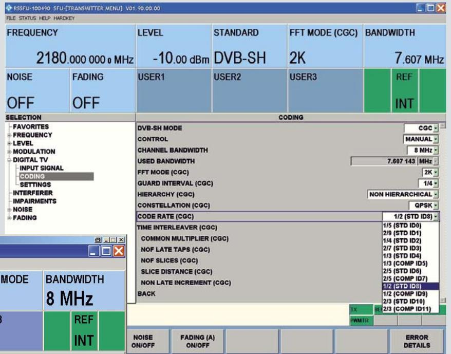
FIG 7 Automatic setting of coding parameters with CMMB.
