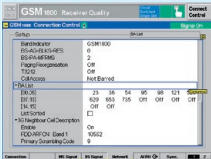
**FIG 2** The mobile phone cyclically determines the receive level on the RF channels listed in the neighbour cell list. The six most powerful RF channels are transmitted from the mobile phone to the base station. The R&S® CMU200 clearly displays these measurement results of the mobile phone.
