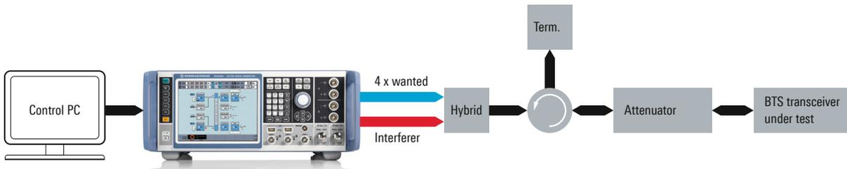
Providing all wanted and interferer signals out of one box makes the two-path R&S®SMW200A with its extensive baseband capabilities an efficient solution for GSM/EDGE AM suppression conformance tests.
