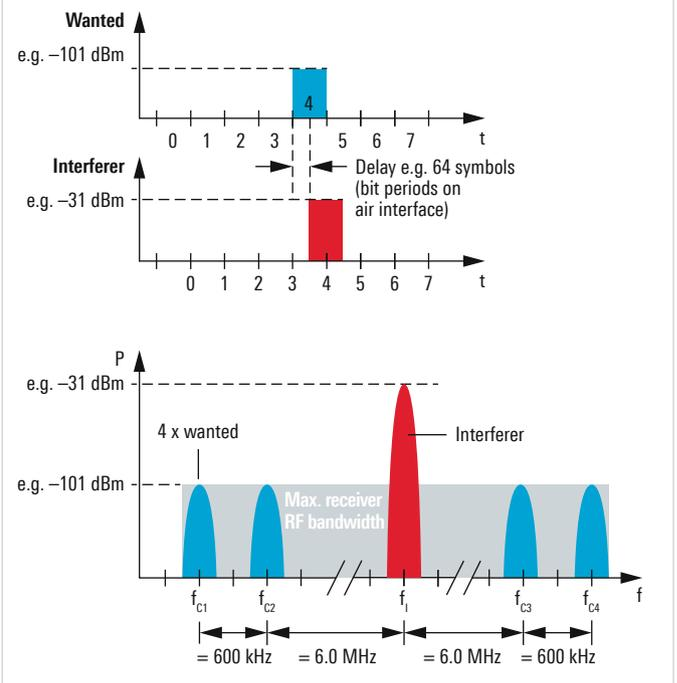
Several properly synchronized vector signal generators (VSGs) provide the required wanted signals to the receiver under test at a certain power level and frequency. An additional VSG delivers the specified modulated interfering signal (at a significantly higher power level) to the receiver.
