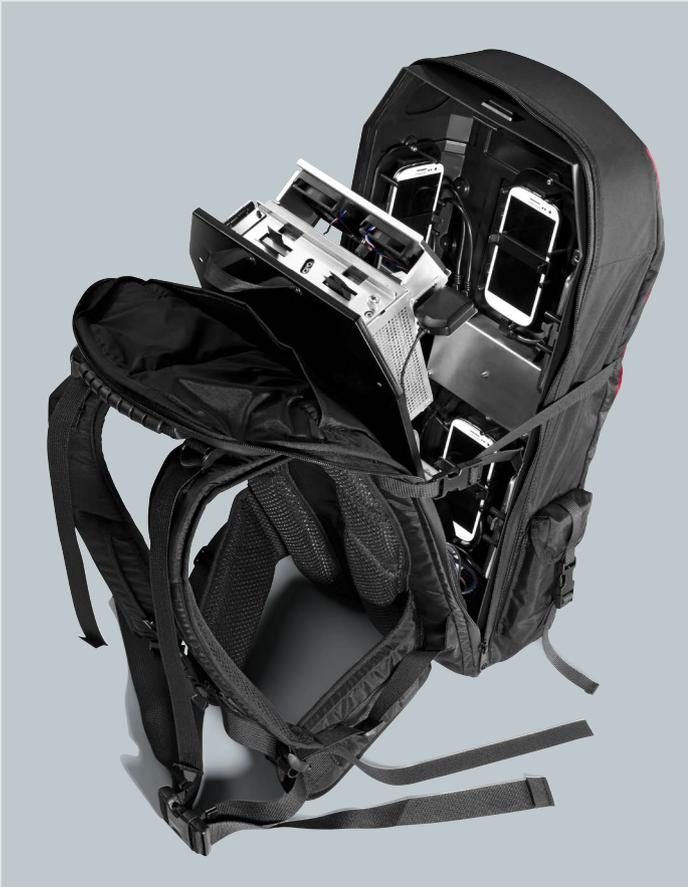
The QualiPoc Freerider is conveniently operated from a tablet that also stores and processes measurement data. The system can record up to six QualiPoc smartphones and two RF scanners (2x2 MIMO), enabling simultaneous measurement of all receivable networks, wireless communications standards and local RF conditions. The instrument's power supply, ventilation and weather protection are designed to make it possible to work a full day under any environmental conditions.
