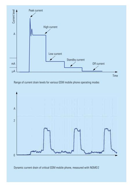
means that this small power supply unit can be used to form the basis of an independent parameter test setup for semiconductor components. The NGMO2 can also handle up to four relays and respond to remote control commands. As each channel has an inhibit input, if required, a pulsed supply voltage can be fed to the components to prevent overheating during tests or to simulate a standard pulsed operating mode (e.g. TDMA power amplifier).
