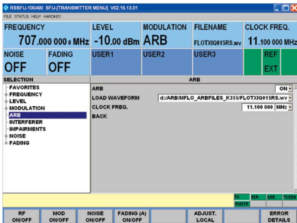
Waveform files are easy to use with instruments from the R&S®SFx family (here R&S®SFU).
