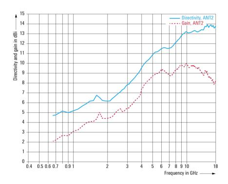
Directivity and gain of the R&S®TC-TA18 cross-polarized Vivaldi test antenna; port ANT2 (meas.).
