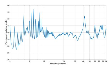
Port-to-port isolation of the R&S®TC-TA85CP cross-polarized Vivaldi test antenna (meas.).
