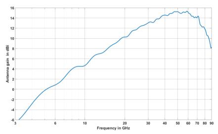
Antenna gain of the R&S®TC-TA85LP linear-polarized Vivaldi test antenna (meas.).
