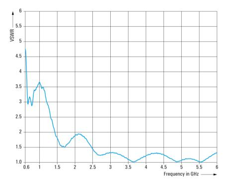
VSWR of the R&S®TC-CA6 linear-polarized communications antenna (meas.).
