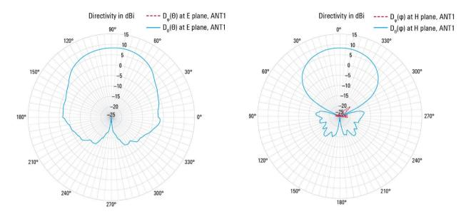
Partial directivity of the R&S®TC-TA18 cross-polarized Vivaldi test antenna at 3 GHz; port ANT1 (meas.).
