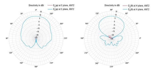
Partial directivity of the R&S®TC-TA18 cross-polarized Vivaldi test antenna at 3 GHz; port ANT2 (meas.).
