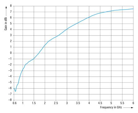
Gain of the R&S®TC-CA6 linear-polarized communications antenna (meas.).
