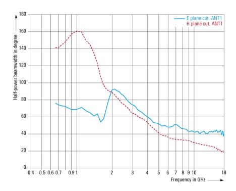
Half-power beamwidth of the R&S®TC-TA18 cross-polarized Vivaldi test antenna; port ANT1 (meas.).
