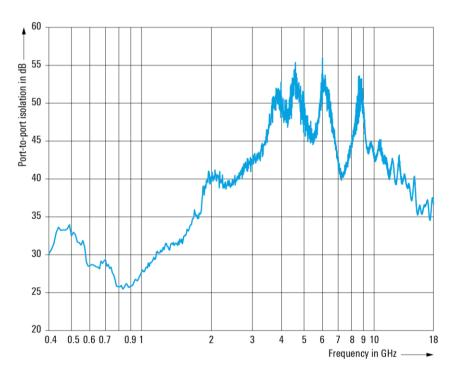
Port-to-port isolation of the R&S®TC-TA18 cross-polarized Vivaldi test antenna (meas.).
