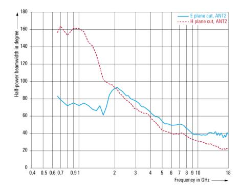
Half-power beamwidth of the R&S®TC-TA18 cross-polarized Vivaldi test antenna; port ANT2 (meas.).
