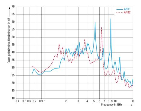
Cross-polarization discrimination of the R&S®TC-TA18 cross-polarized Vivaldi test antenna (meas.).
