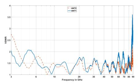
VSWR of the R&S®TC-TA85CP cross-polarized Vivaldi test antenna (meas.).
