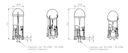
Dimensions of the R&S®TC-TA85CP cross-polarized (left) and the R&S®TC-TA85LP linear-polarized (right) Vivaldi test antennas.
