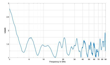
VSWR of the R&S®TC-TA85LP linear-polarized Vivaldi test antenna (meas.).
