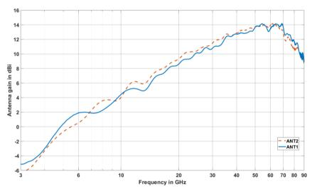
Antenna gain of the R&S®TC-TA85CP cross-polarized Vivaldi test antenna (meas.).
