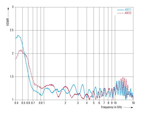
VSWR of the R&S®TC-TA18 cross-polarized Vivaldi test antenna (meas.).
