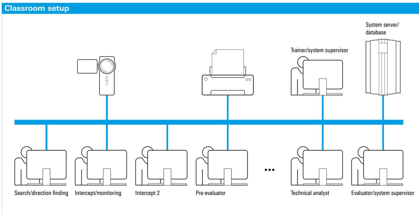
R&S®SRTS in a classroom setup with various trainee workstations, the central system server for hardware and software simulation, the trainer's workstation and a projector for the trainee workstations to evaluate the training.
