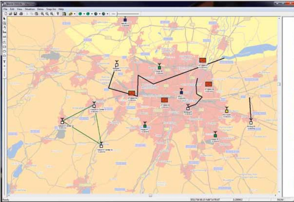
Display of the current signal scenario in R&S®MapView. The symbols indicate the positions of the transmitter stations. It is also possible to define transmitter routes on which the transmitters move at the speed specified by the trainer.
