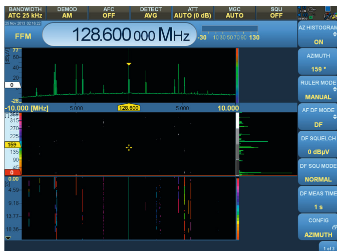
R&S®DDF255 graphical user interface displaying 20 MHz realtime bandwidth.
