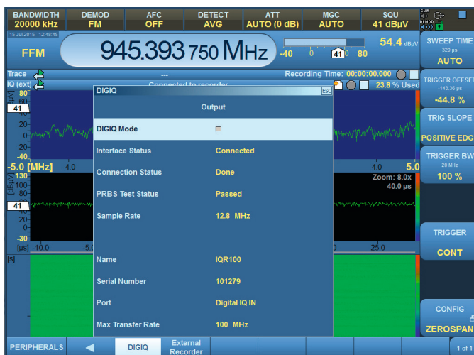
Status report for an R&S®IQR100 connected to the R&S®Digital I/Q Interface.
