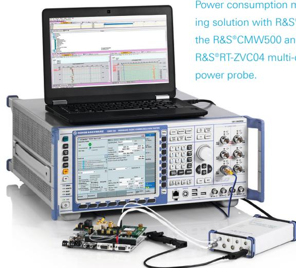
Power consumption monitoring solution with R&S®CMWrun, the R&S®CMW500 and the R&S®RT-ZVC04 multi-channel power probe.
