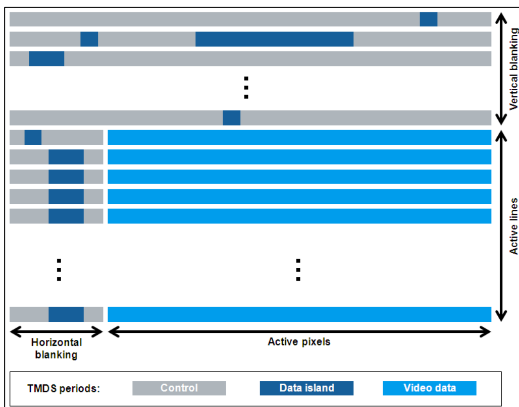
Fig. 4: Transmission structure of the TMDS channel
