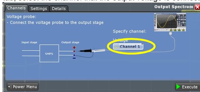
Figure 21: Output spectrum “Channels” tab
