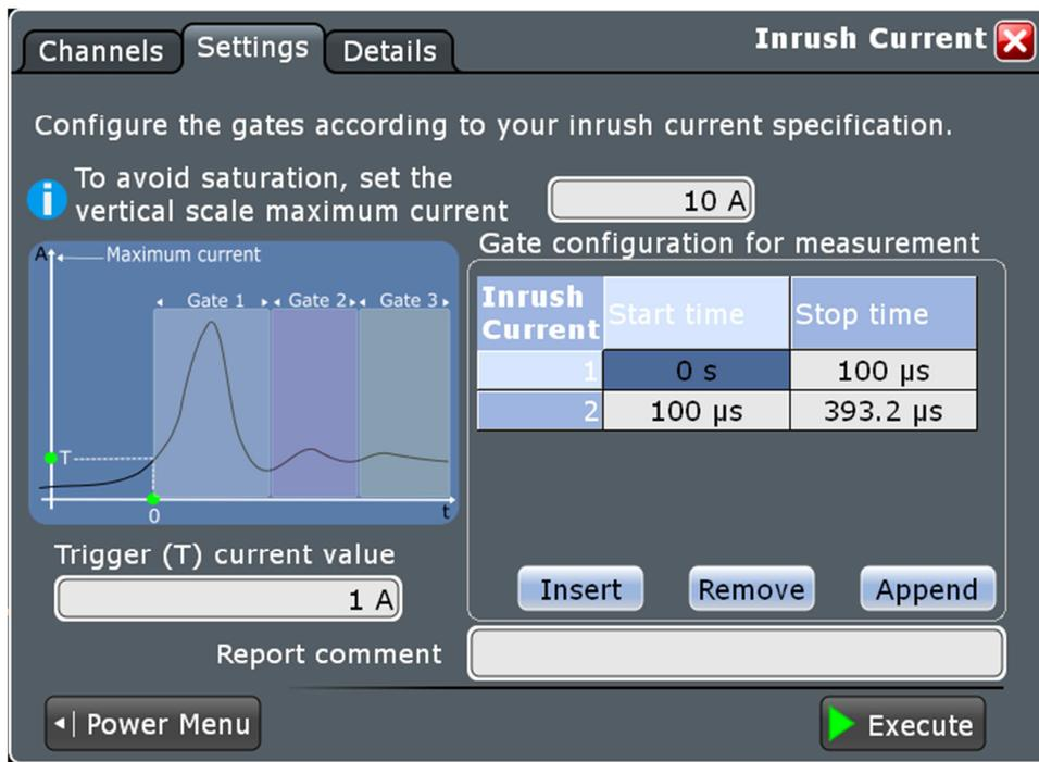
Figure 14: Setting options for the Inrush Current measurement
