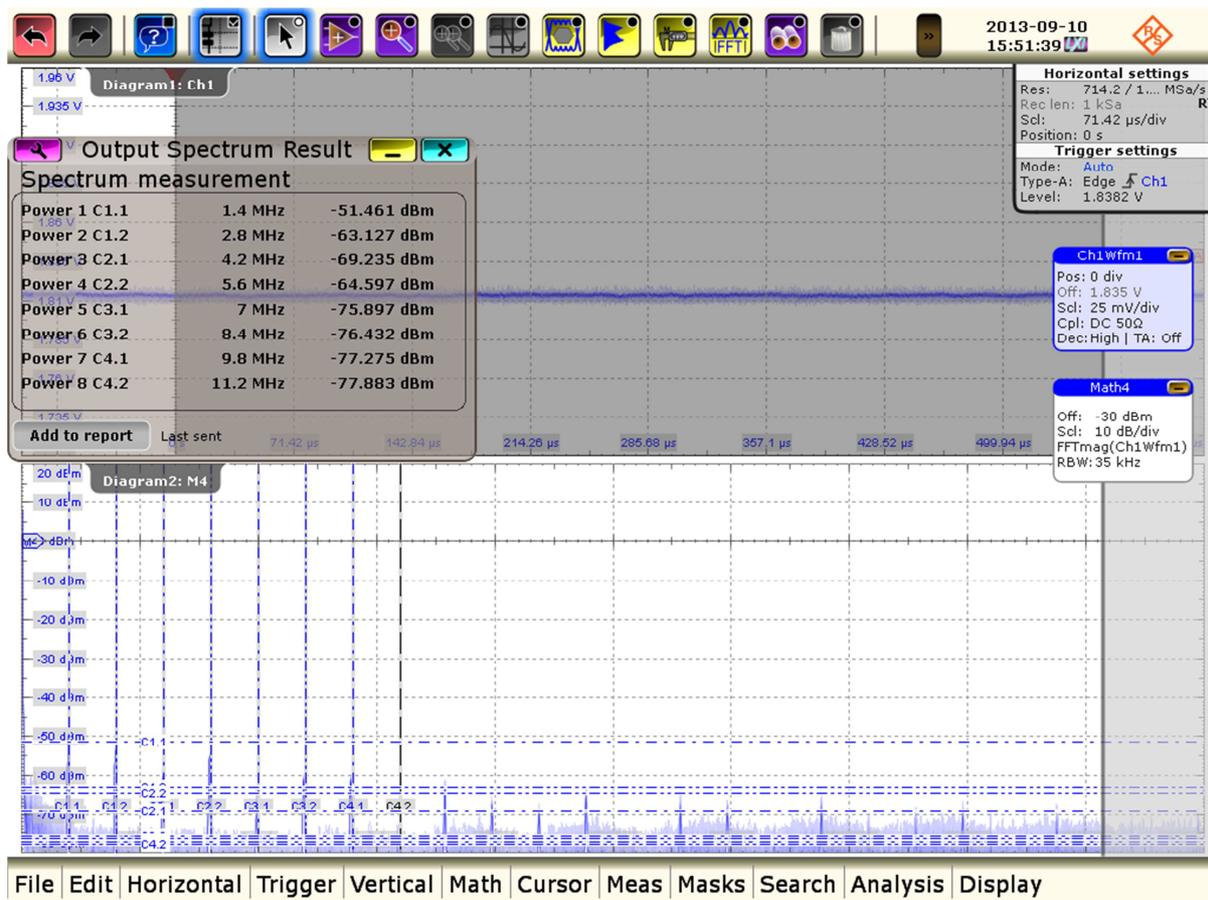
Figure 23: R&S®RTO-K31 Output ripple spectrum auto-scaled measurement display
