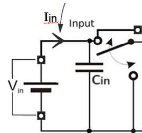
Figure 13: Current probe point for DC/DC converter Inrush Current measurement
