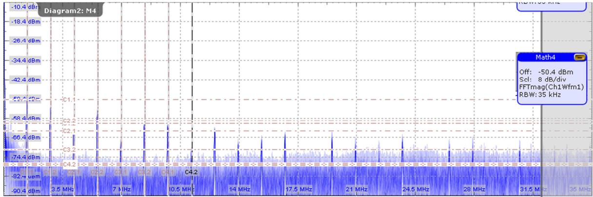
Figure 24: Output spectrum display with manual adjustment of gain and offset
