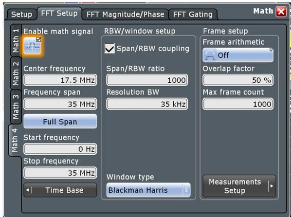
Figure 27 Math channel FFT Setup for output ripple spectrum
