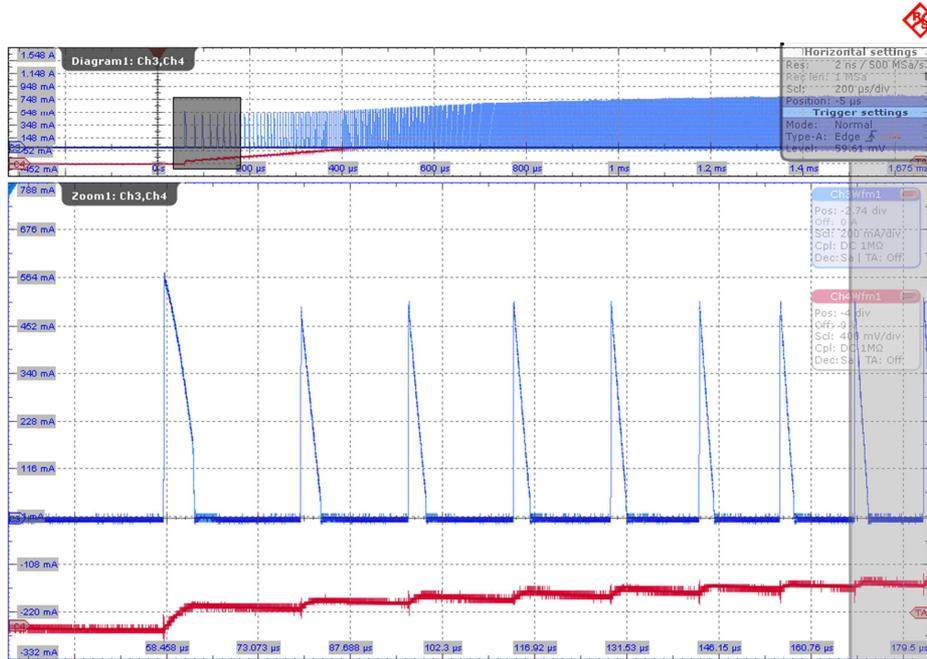
Figure 8: TPS62090 Soft-start at 10% load  $V_{in} = 5\text{ V}$ ; Zoom of first few cycles (Ch 4 red -  $V_{out}$  / Ch 3 blue -  $I_{in}$ )
