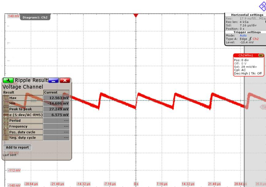
Figure 19: R&S®RTO-K31 Output ripple measurement screen
