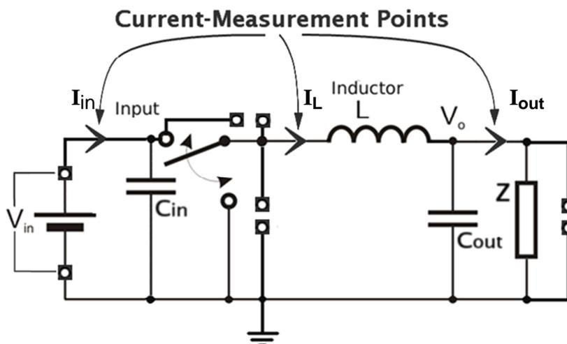
Figure 3 Important current measurement points
