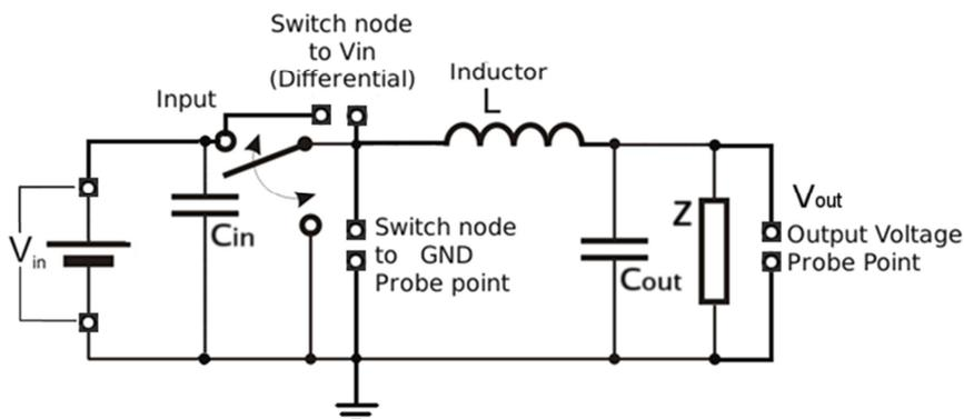
Figure 2 Overview of probing points for voltage measurements on a DC/DC buck converter
