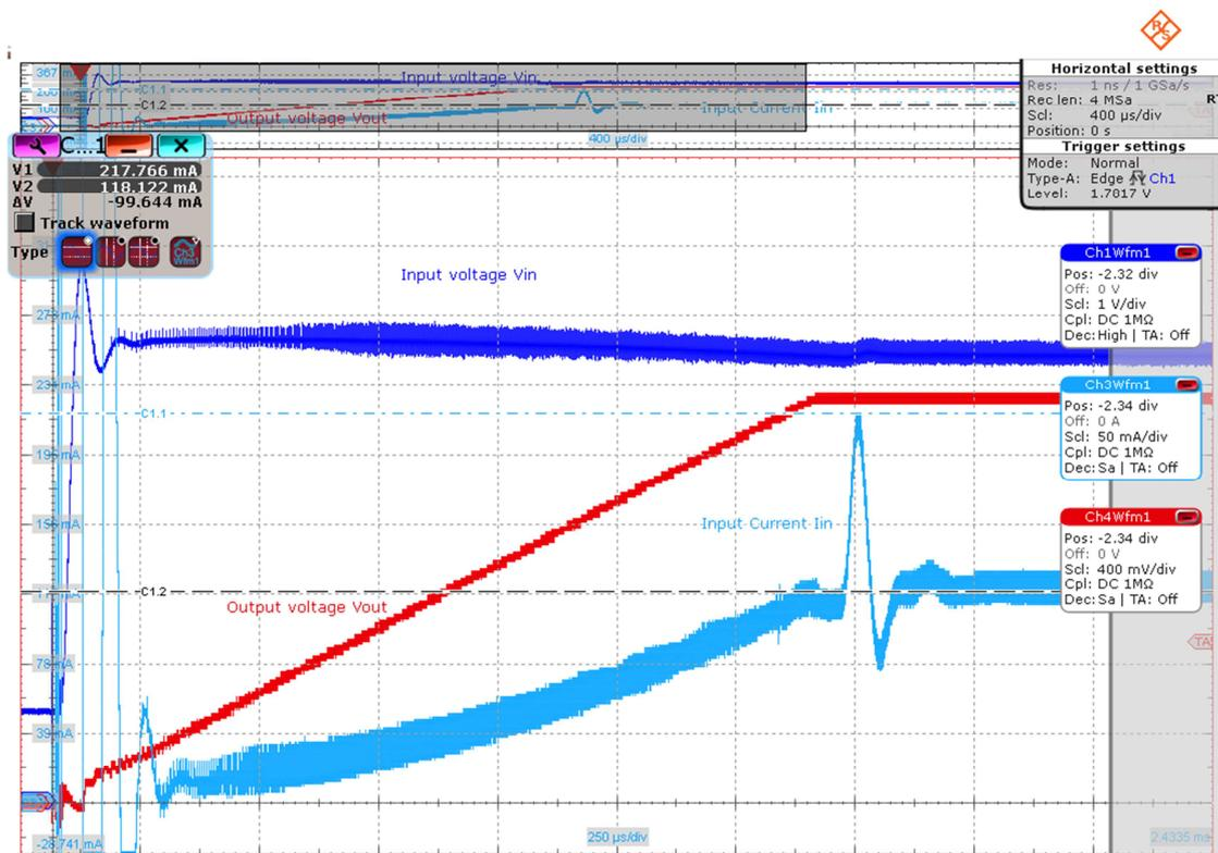
Figure 7: TPS62090 Soft-start at 10% load  $V_{in} = 5\text{ V}$
