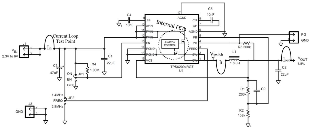
Figure 4: TPS62090 EVM simplified schematic, showing added current and voltage test points
