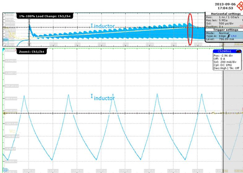
Figure 17: A different controller IC and components, showing distorted inductor-current waveforms, at peak inductor current (red oval indicates the zoomed area.) (Ch 3 light blue - Iin)
