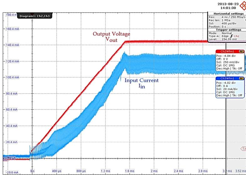
Figure 16: Start-up of DC/DC converter, showing inductor current peak at the end of the soft-start period (Ch 2 red - Vout / Ch 3 light blue - Iin)
