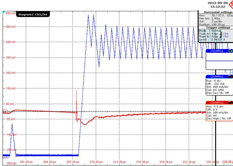
Figure 18: A 1% - 100% load step of TPS62090 showing no apparent distortion of inductor-current waveform at peak current of transition (Ch 4 red - Vout / Ch 3 light blue - Iin)
