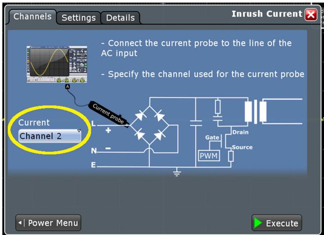
Figure 12: Channels Tab for Inrush Current setup
