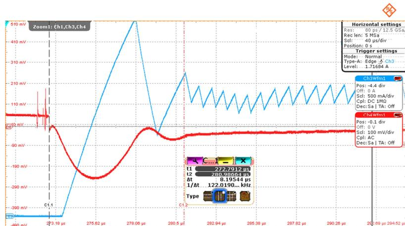
Figure 30: 1% to 100% load change TPS62090 with  $V_{in} = 3.3\text{ V}$ ; approximately  $9\ \mu\text{s}$  to begin full regulation. Note the higher current peak and duty-cycle difference versus the 5 V test result of Figure 29.
