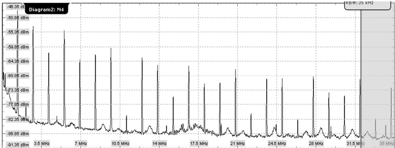
Figure 28 Output ripple spectrum display with waveform averaging over 20 measurements
