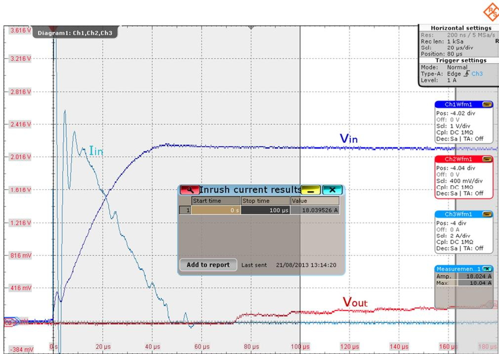
Figure 15: Start-up waveforms and result table of the Inrush Current measurement function;  $V_{switch}$  is not shown, as its activity, at this horizontal scale, appears to be a solid 'wall' from ground to  $V_{in}$ .
