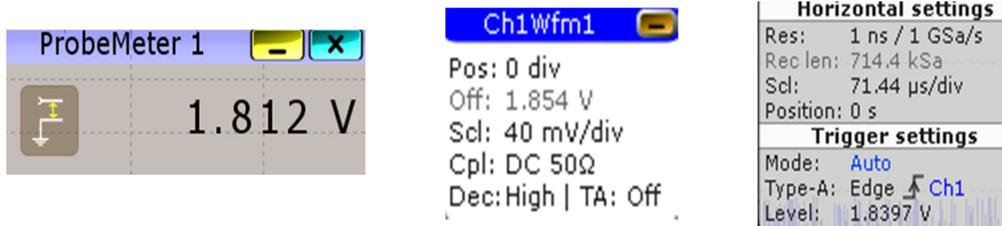
Figure 25: Oscilloscope settings to observe output ripple
