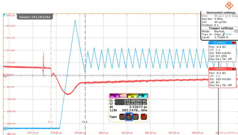
Figure 29: 1% to 100% load change TPS62090 with  $V_{in} = 5\text{ V}$ ;  $< 4\ \mu\text{s}$  to begin full regulation.
