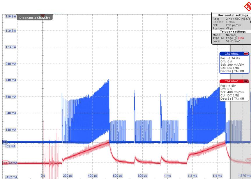
Figure 9: TPS62090 does not start with heavy loads below 0.8 V (Ch 4 red -  $V_{out}$  / Ch 3 blue -  $I_{in}$ )
