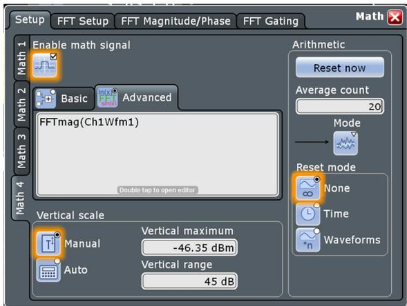
Figure 26 Math channel basic setup for output ripple spectrum
