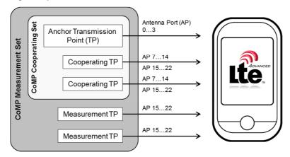
concept of virtual cell identities can be applied. Virtual cell identifies are assigned by higher layer.
