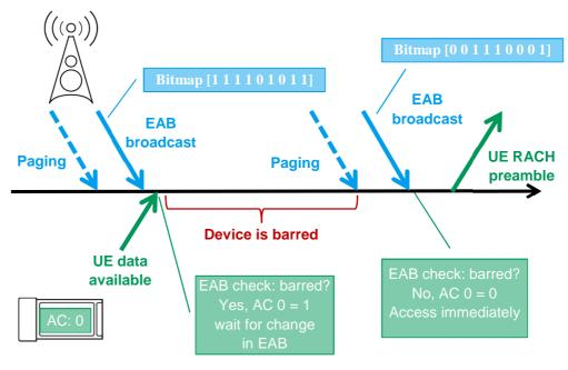
Fig. 2-21: EAB principle
