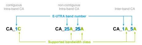
Fig. 2-3: Notation of carrier aggregation support (type, frequency band, and bandwidth)
