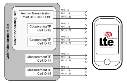
Fig. 2-7: Downlink CoMP Cooperating and Measurement Set for cells using *different* cell identities.
