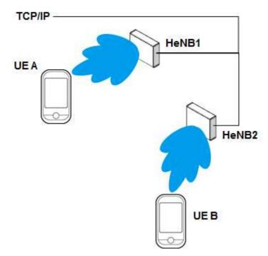
Fig. 2-9: Example of Coordinated Scheduling / Beamforming (CBS) with two femto cells
