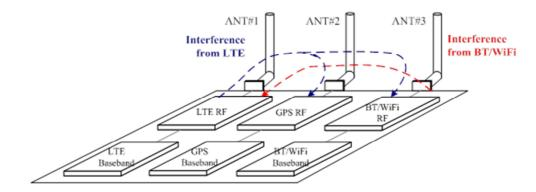
Fig. 2-19: Example implementation of LTE, GPS and WiFi in a single device
