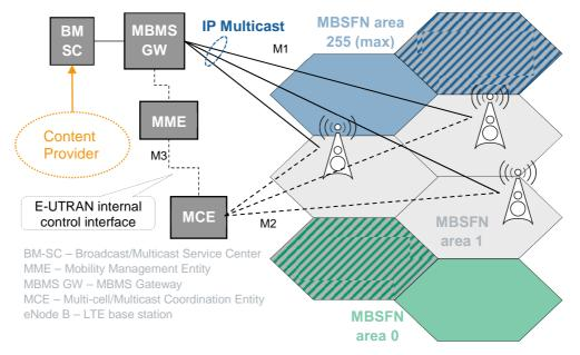
Fig. 2-17: MBMS architecture and interfaces
