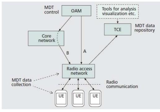
Fig. 2-22: Measurement control of MDT by the OAM. Path A denotes the management-based MDT, path B the signaling-based MDT (source [16]).
