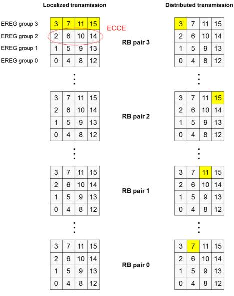
Fig. 2-15: E-PDCCH – Localized versus Distributed Transmission
