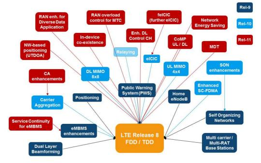
Fig. 1-1: 3GPP Release 8 to 11 technology component dependencies
