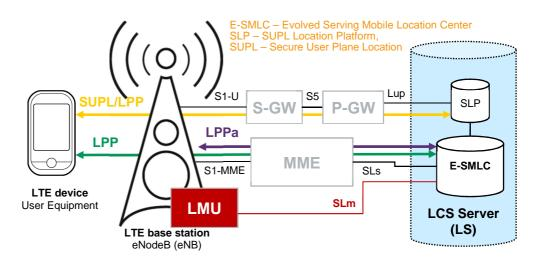
Fig. 2-16: E-UTRA supported positioning network architecture
