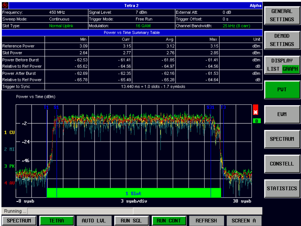
Figure 8: Analysis of a TETRA Release 2 signal using the R&S®FS-K110 option. The green bar marks the signal section which is used to derive the numerical results. It is positioned automatically.
