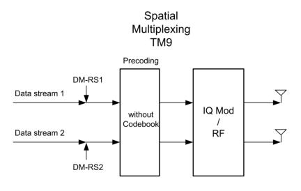
Figure 20: TM9: The UE-specific RS is applied before the precoding. This enables non-codebook based precoding. So the full range of beamforming patterns can be used.
