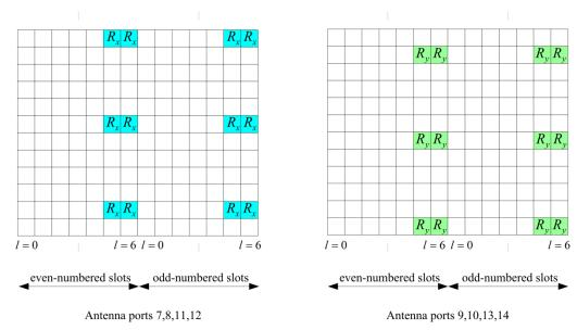
Figure 18: Distribution of reference signals for transmission mode 9 (antenna ports 7...14) [1]
