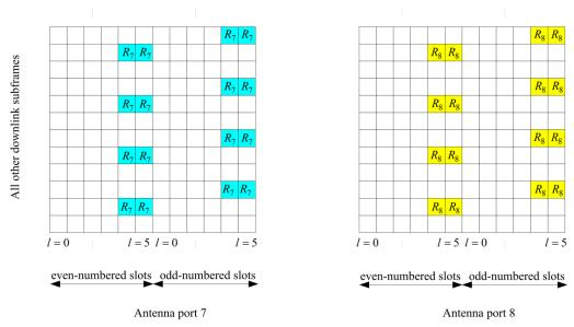
Figure 15: Distribution of reference signals for transmission mode 8 (antenna ports 7 and 8) [1]
