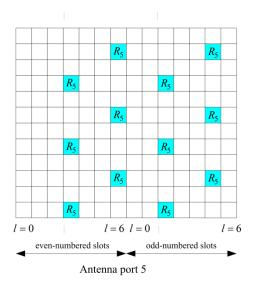
Figure 7: Distribution of reference signals for transmission mode 7 [1]
