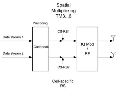
Figure 19: TM3...6: The cell-specific RS is applied after the precoding. The UE reports back the wanted codebook index. Only discrete beamforming patterns are used (see 3.2.4 and 3.2.6).
