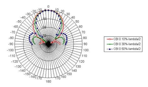
Figure 4: The antenna diagram is affected by the distance d between the antennas. In this example, d is 10 %, 30 %, and 50 % greater than N2. (CBI 0 refers to code book index 0, see chapter 3.2.4)
