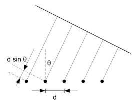
Figure 2: Antenna array with a distance d between the individual antennas. The additional path that a wavefront must traverse between two antennas is d \*  $\sin \theta$ .
