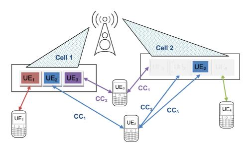
Figure 4: LTE-Advanced maximum bandwidth in contiguous deployment
