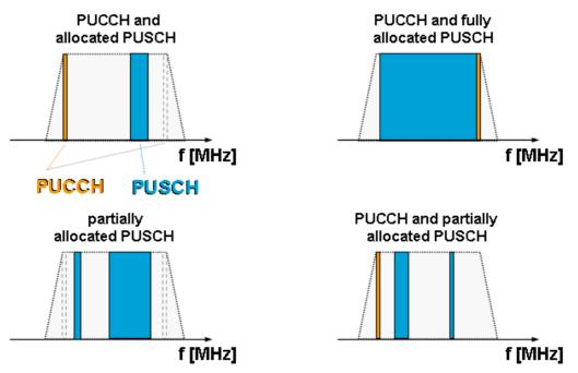
Figure 16: PUSCH and PUCCH combinations in 3GPP Release 10
