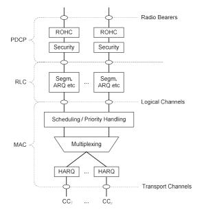
Figure 12: Uplink layer 2 structure [3]
