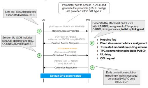
Figure 2: LTE attach procedure
