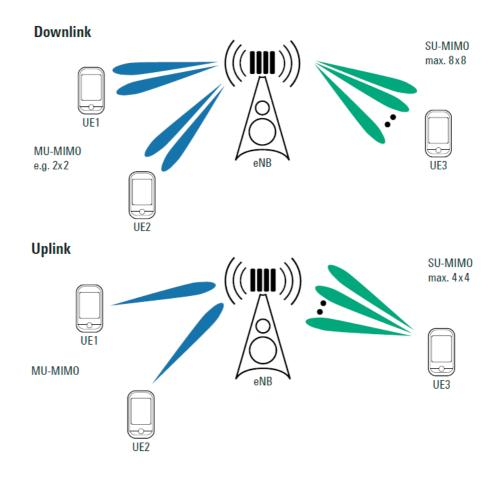
Figure 14: Supported transmit layers in LTE-Advanced
