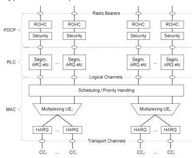
Figure 11: Downlink layer 2 structure [3]
