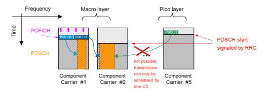
Figure 10: Cross carrier scheduling for support in heterogeneous networks
