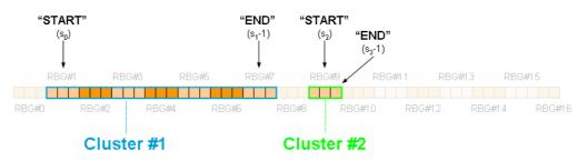
Figure 18: Example for a two-cluster allocation for a 10 MHz (50 RB) signal
