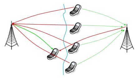
Figure 19: Interference scenario in a macro cell network
