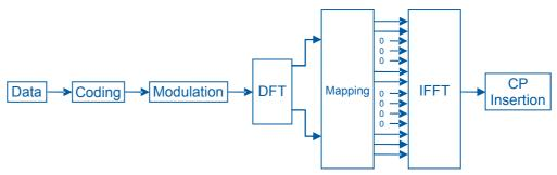
Figure 17: Block diagram for clustered SC-FDMA
