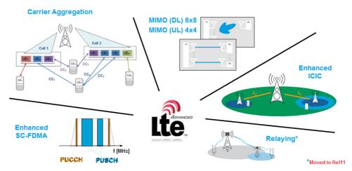
Figure 1: Main LTE-Advanced technology components (overview)
