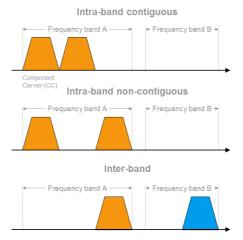
Figure 6: LTE-Advanced spectrum deployment
