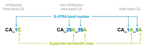
Figure 8: Notation of carrier aggregation support (type, frequency band, and bandwidth)
