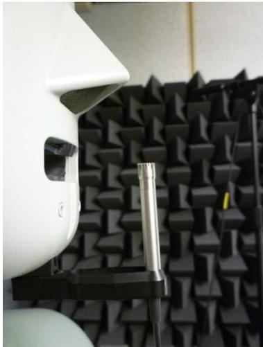
Fig. 2-8: Position of the reference microphone for calibration of the HATS artificial mouth
