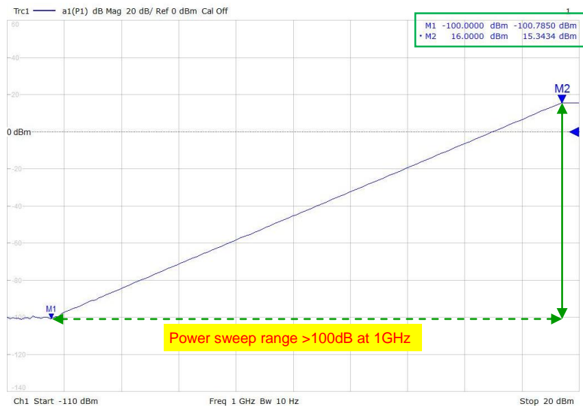
Figure 10 – Power sweep characteristic of R&S® ZNB analyzer
