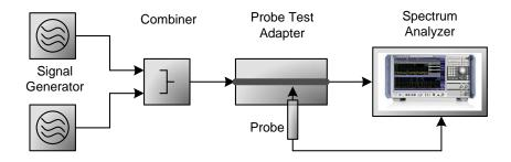
Fig. 3-2: Block circuit of intermodulation distortion test setup
