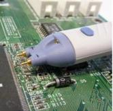
Fig. 2-7: Examples for a differential probe directly connected to a circuit
