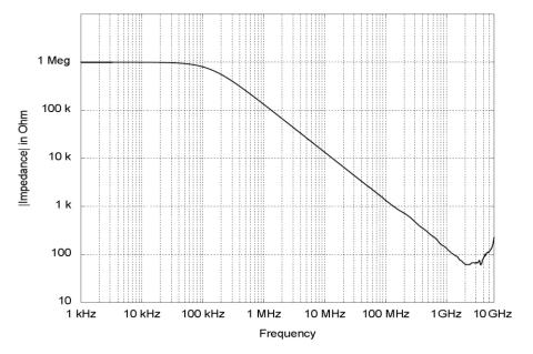
Fig. 2-2: Plot of the Input Impedance versus frequency for active probe R&S RT-ZS30
