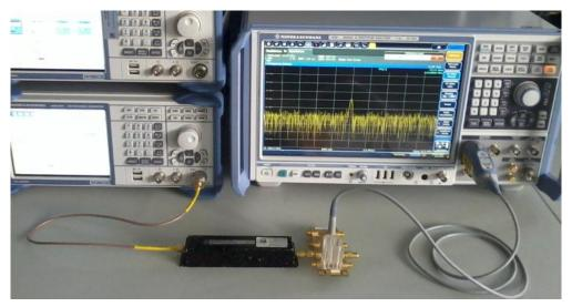
Fig. 3-5: Test setup for harmonic distortion test for RT-ZS30at 100 MHz
