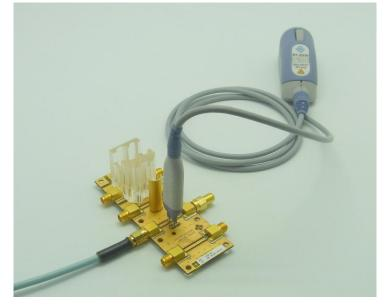
Fig. 3-1: Probe test adapter used for performance evaluation
