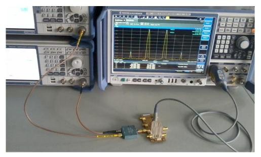
Fig. 3-3: Test setup for intermodulation distortion test of the RT-ZS30 at 500 MHz
