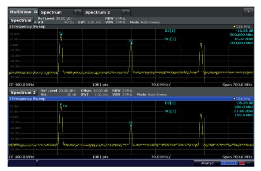
Fig. 4-2: Test result of the differential amplifier connected to the spectrum analyzer
