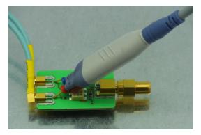
Fig. 4-3: Differential Probe connected to output circuit
