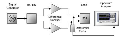
Fig. 4-1: Block circuit of the differential amplifier test setup
