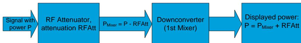
**Figure 4: Signal Power Flow Chart through a Spectrum Analyzer, with signal power  $P$ , RF attenuation setting  $RFAtt$ , signal power at mixer  $P_{Mixer}$ , and displayed Power  $P (= \text{signal power})$**
