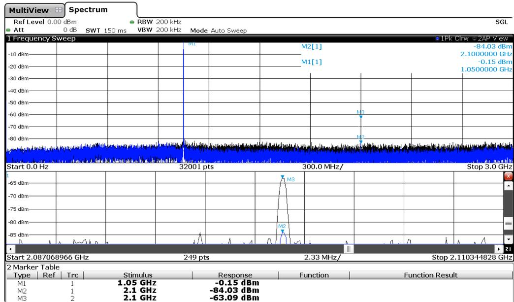
Figure 6: Fundamental and second harmonic, black trace with High Pass Filters Off, blue trace with High Pass Filters On, same RF attenuation. The lower diagram shows the zoomed area around the 2<sup>nd</sup> harmonic.
