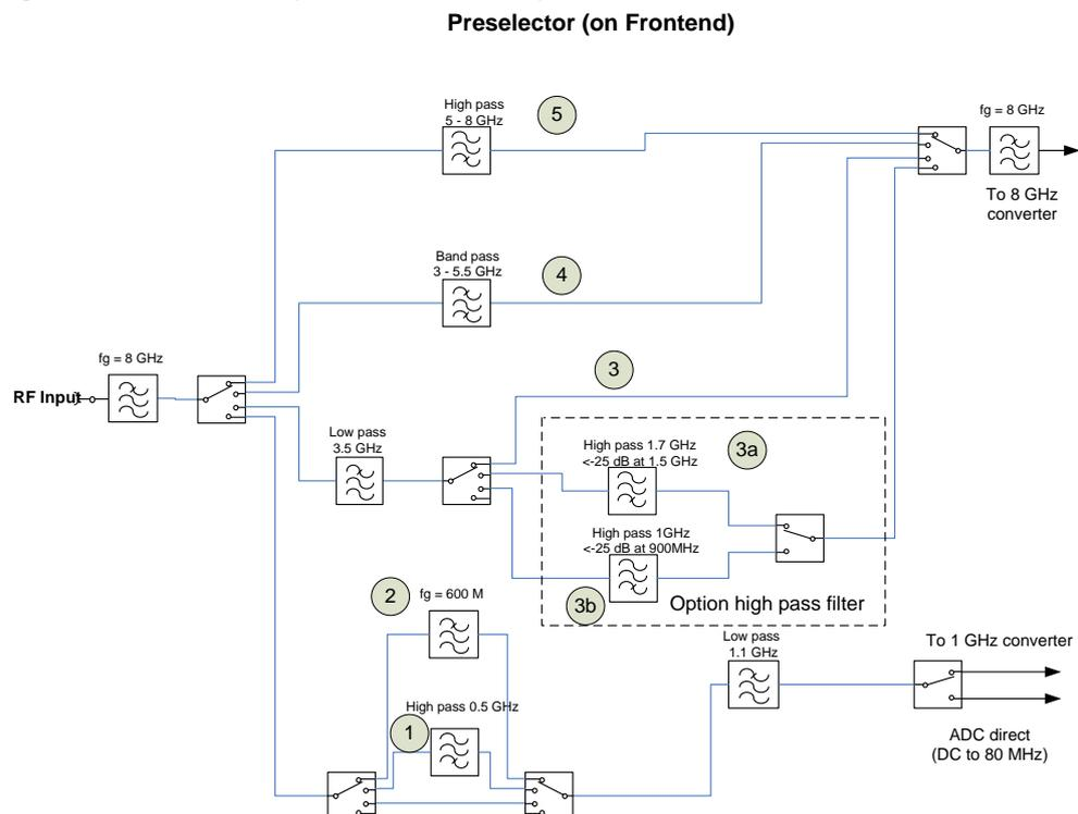
**Figure 3: Signal Flow for  $f \leq 8$  GHz**
