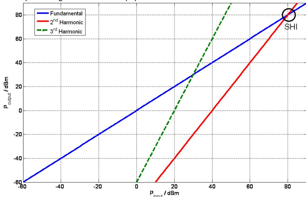
Figure 1: Input and output levels of a non-linear element with gain 1, for fundamental, 2<sup>nd</sup> and 3<sup>rd</sup> harmonics, single tone scenario
