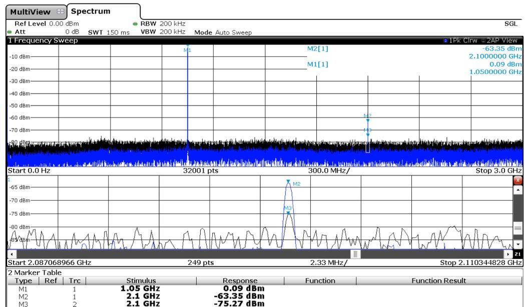
**Figure 5: Fundamental and second harmonic, black trace with 10 dB RF attenuation, blue trace with 0 dB. The lower diagram shows the zoomed area around the 2<sup>nd</sup> harmonic**
