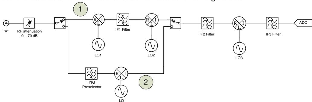
**Figure 2: Simplified block diagram of a heterodyne spectrum analyzer, with RF path "1", and microwave path "2"**
