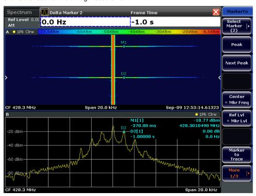
Fig. 4-5: Timing measurement with split screen spectrogram and real-time spectrum
