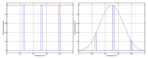
Fig. 2-3: Pulse signal in time domain. Different window functions are applied to the same signal: left - rectangular - no weighting, right - Blackman - pulses on the right and left are highly attenuated
