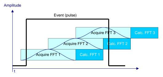
Fig. 2-10: Real-time configuration with overlap; the measured event is longer than the POI time and therefore displayed with 100% true power
