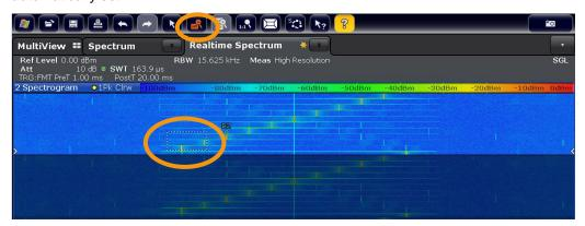
Fig. 2-12: Spectrogram with magnifying tool selected. Light area in spectrogram indicates zoom able area, dark area: not zoom able
