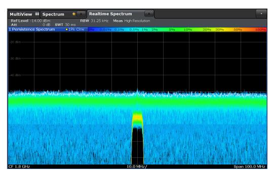
Fig. 4-7: Wideband noise-like signal covering a WCDMA signal
