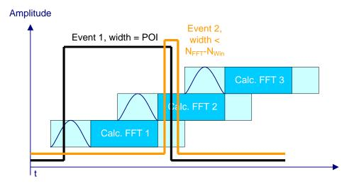
Fig. 2-11: Real-time configuration with no overlapping; event is short enough so it can completely disappear between two consecutive window functions
