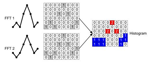
Fig. 4-8: Schematic of histogram calculation (dot style)
