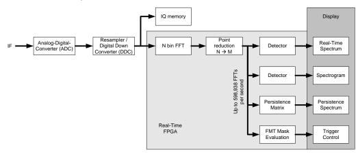
Fig. 2-1: Signal flow chart of the digital real-time part of the Rohde & Schwarz real-time analyzers
