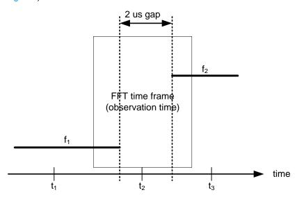
Fig. 2-8: Timing diagram of the FFT observation time example
