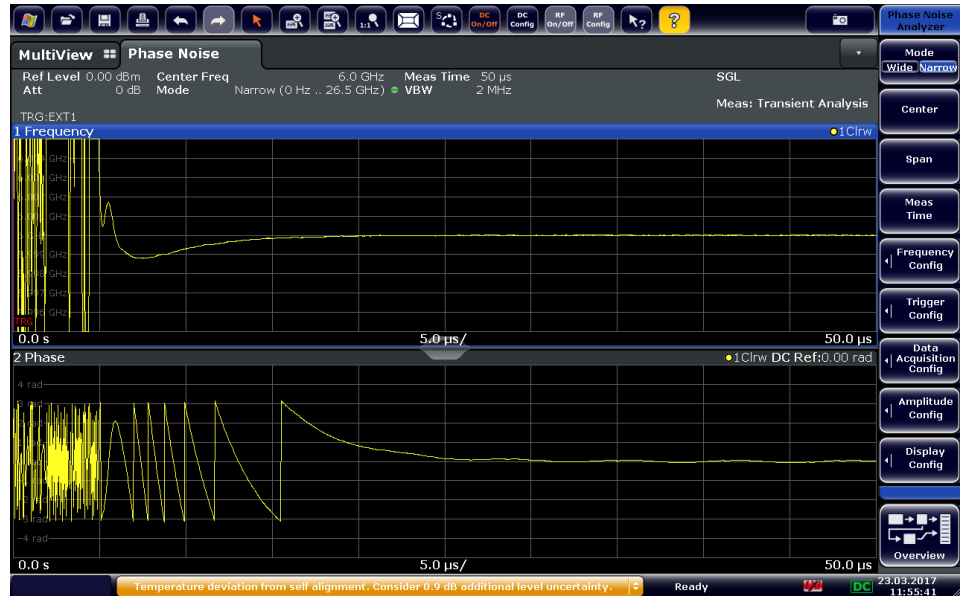
Fig. 4.2-1: Frequency and phase settling time measurement in parallel
