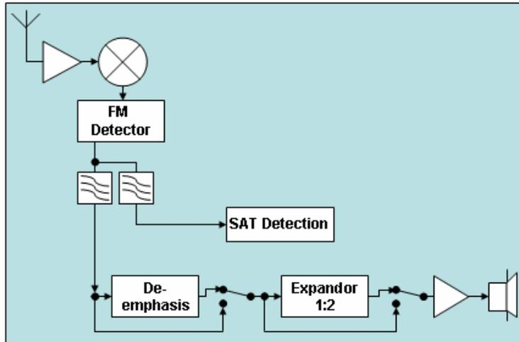
The RF signal is mixed with the baseband and is passed on to an FM detector. Depending on the “SAT Color Code (SCC)”, the signal components “voice” (300 Hz to 4 kHz) and “Supervisory Audio Tone” (5970 Hz, 6000 Hz or 6030 Hz) are filtered out of the demodulated signal.
