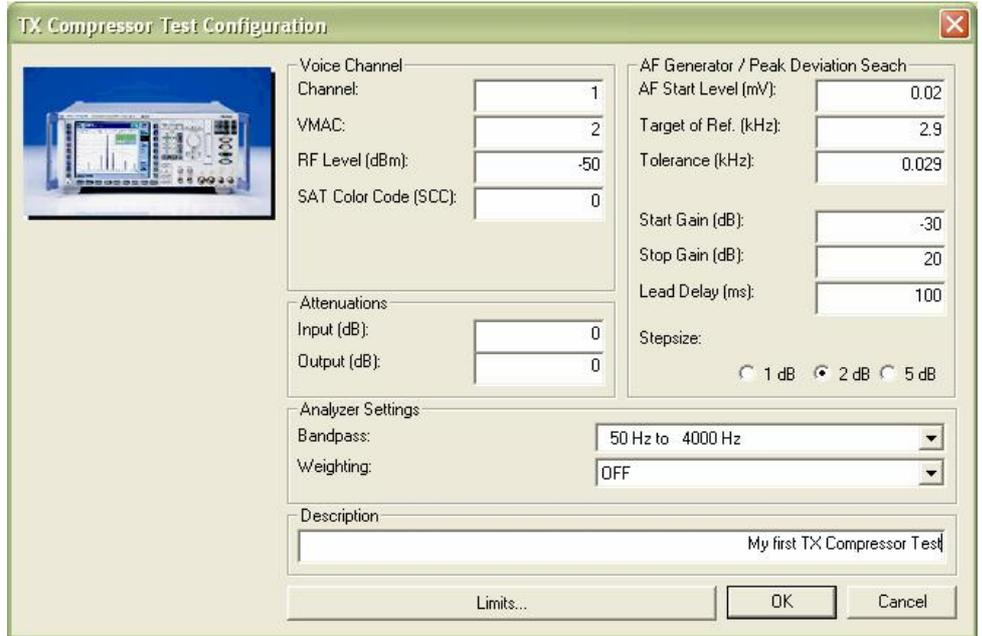
The purpose of this test is to measure the compressor of the AMPS phone. You have to enter the following parameters for this test:
