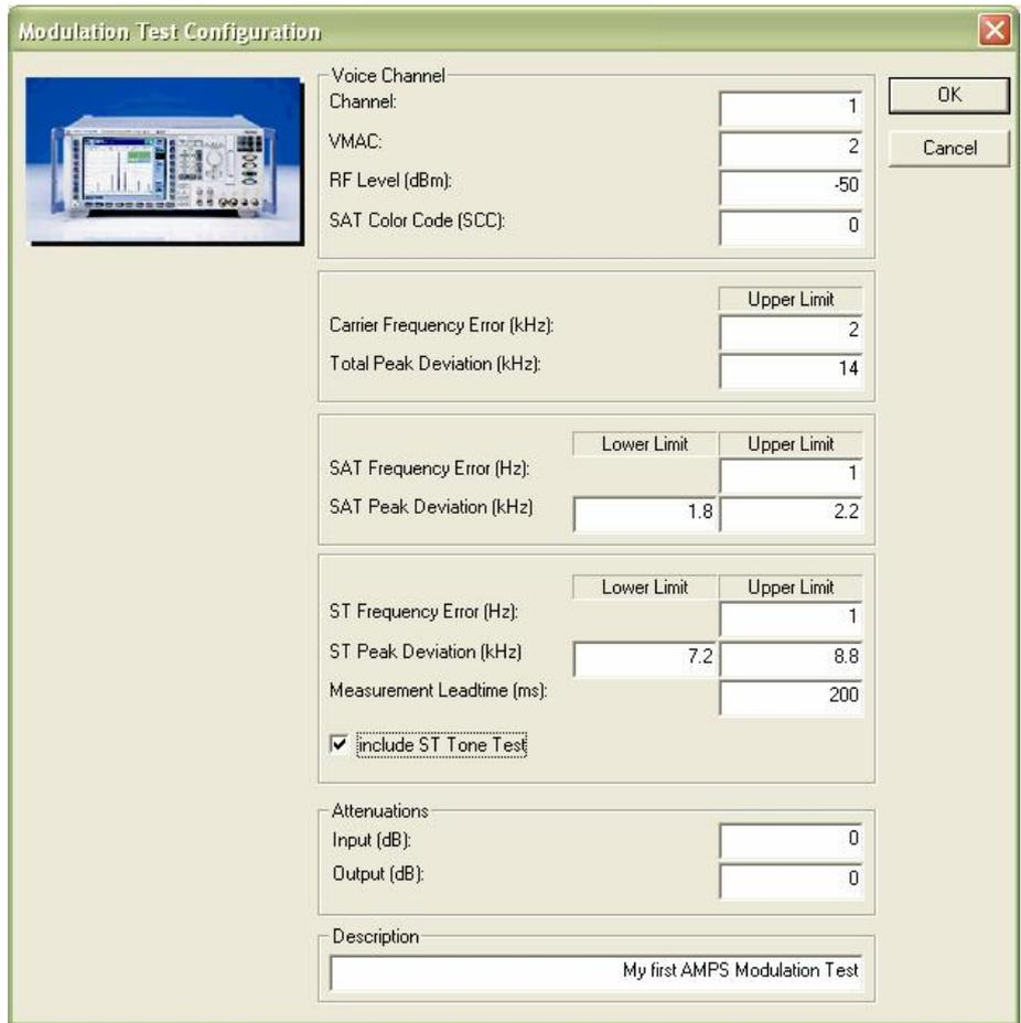
The purpose of this test is to test the frequency error of the phone and to check whether the modulation deviation for the voice signal, SAT and ST is correct. You have to enter the following parameters for this test:
