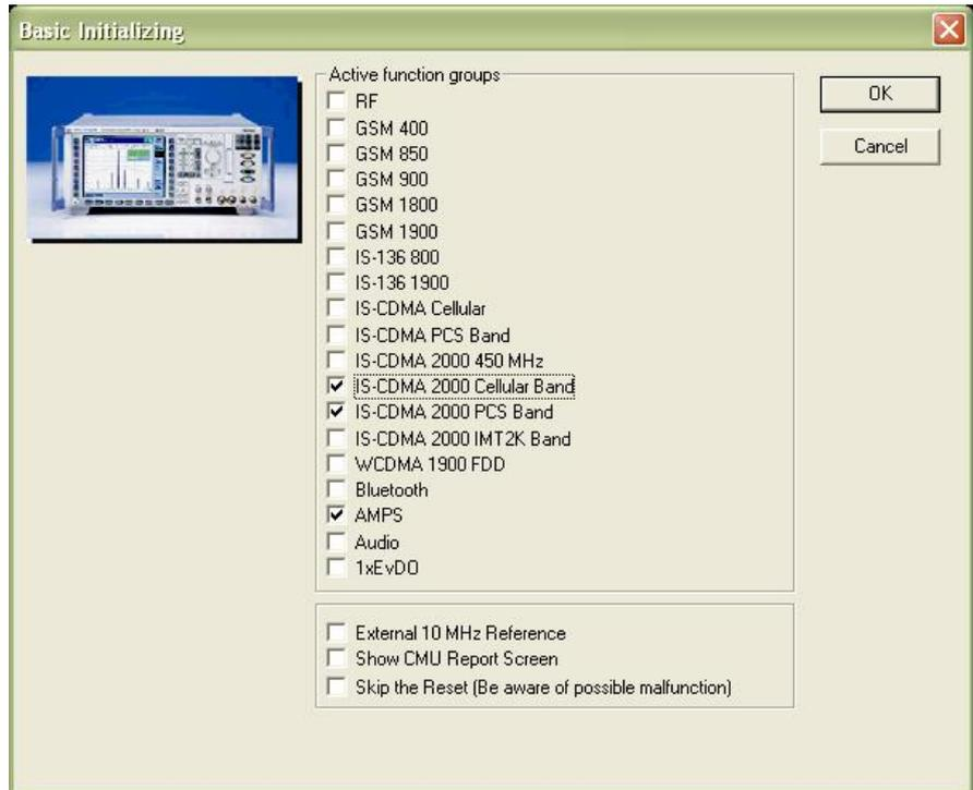
“Basic Initializing” is always at the beginning of a remote-control sequence. In this test item the available CMU options are queried and “address mapping” (i.e. the assignment of the individual secondary addresses to the respective function groups) is performed.
