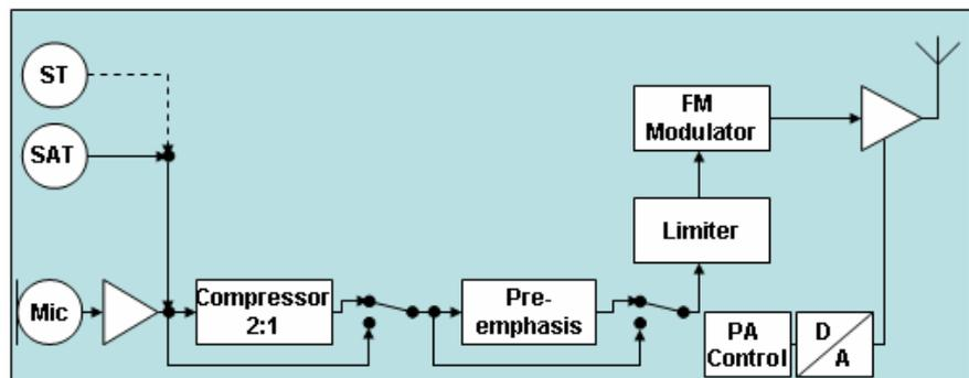
In the AMPS phone, the amplified audio signal from the microphone first enters a “compressor”. The reference deviation for AMPS is 2.9 kHz. This means that the audio signal should generate a deviation of 2.9 kHz at full-scale level. The relationship between audio signal level and deviation is, however, not linear. A 6-dB-lower input level attenuates the deviation by only 3 dB. A 6-dB-higher audio signal amplifies the deviation by only 3 dB.
