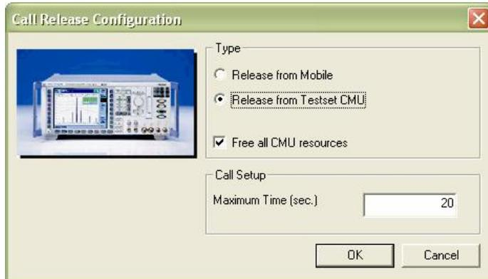
The following parameters are specified when configuring the test:
