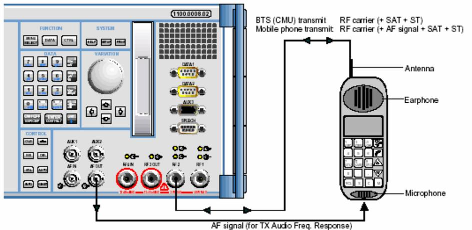
RF2 is normally used for the bidirectional RF connection. It is also possible to use the RF1 connector; however, the dynamic range of this input (and output) is less suitable for testing AMPS phones. There is one exception: if
