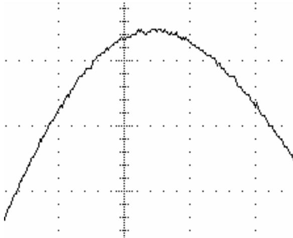
The value to  $\text{RMS} * \sqrt{2}$  yields much more stable values for the level search since it “filters out” any interference. These values are then, however, lower than the displayed peak value. Consequently, the audio level found using the level search is higher than that for instruments which only provide peak weighting.
