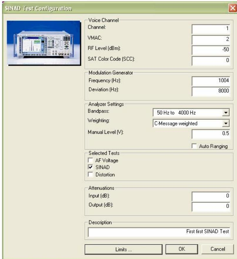
The last RX measurement is the SINAD measurement (signal-to-noise ratio). This test is used to measure the audio distortion of the phone at the loudspeaker output. It is also possible to check whether the output voltage of the audio signal is within the expected range.
