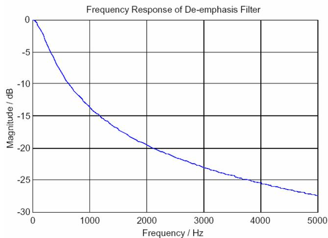
The audio signal is passed on to the “de-emphasis filter” which should cancel out the effect of the “emphasis filter”. The “expander” is next. This is the counterpart of the “compressor”. With an input deviation of 2.9 kHz, the audio reference level thus returns to 0 dB. An input deviation of -3 dB results in an audio signal which is lower than -6 dB. A 3-dB-higher deviation results in a 6-dB-higher output signal.
