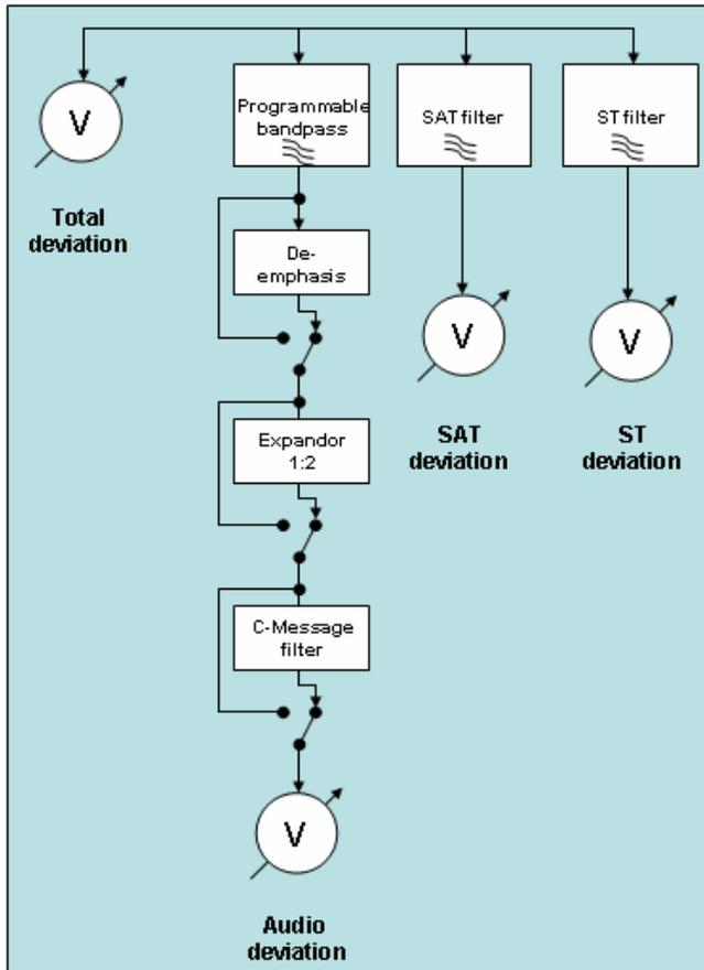
The measuring path of the R&S CMU200 shown in simplified form above is similar in structure to the RX path of the mobile phone. Measurement of the deviation is divided into four components: total deviation, SAT deviation, ST deviation and, of course, audio deviation. The bandpass filter for measuring the SAT is determined automatically according to the set "SAT Color Code (SCC)".
