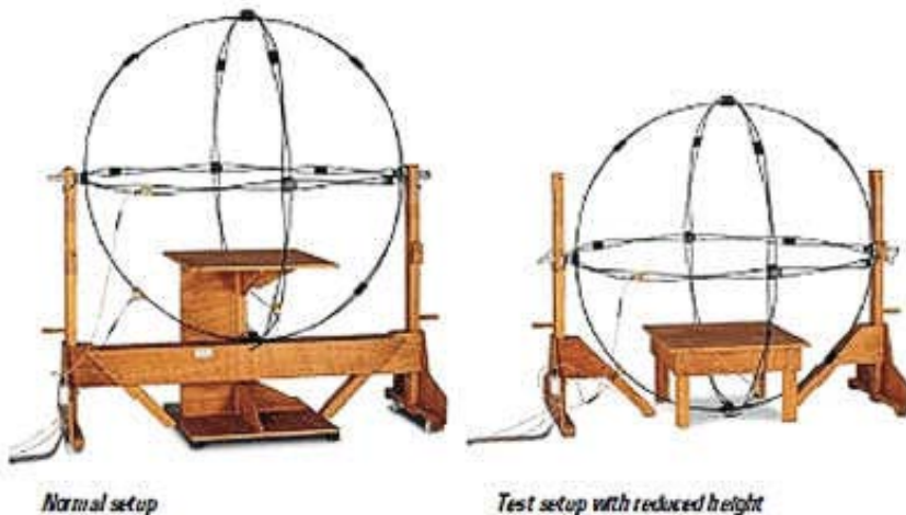
R&S®HM20 triple-loop antenna for lighting equipment emission measurements.
