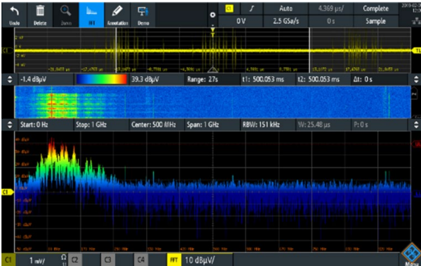
Figure 9: A digital oscilloscope can be used to investigate the correlation between time- and frequency-domain activity.
