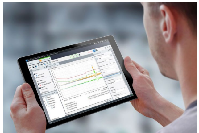
Figure 13: A simplified and dedicated version of the R&S® ELEKTRA software (R&S®ELEMI-E) addresses EMI precompliance testing, covering the most common EMI standards with predefined templates.
