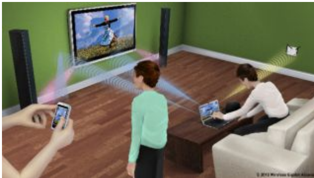
Figure 8: 802.11ad, or WiGig, enables data speeds to almost 7 Gbit/s but requires a direct line of sight between devices.
