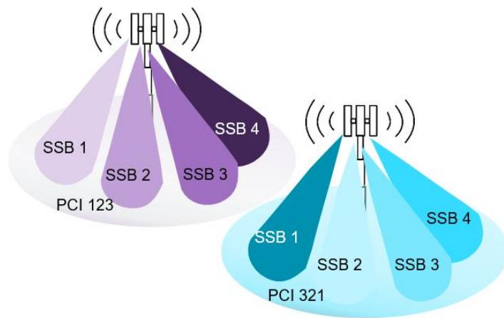
Figure 20: Two 5G NR cells with different PCIs (123, 321) and four SSB beams each
