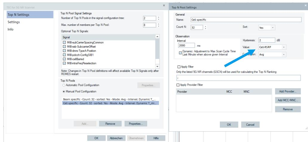
Figure 15: Top N Settings in ROMES4 for a Cell / PCI specific Top N Pool
