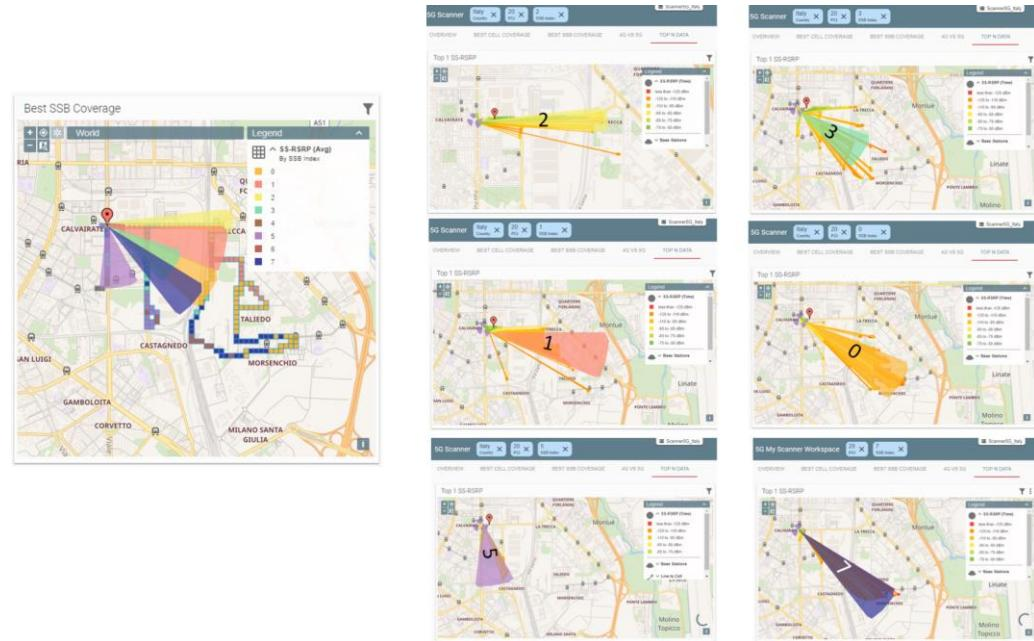
**Figure 58 5G Scanner Beam coverage analysis**
