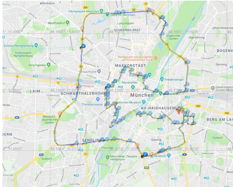
**Figure 40: R&S@ROMES4 Network Problem Analyzer with detected interference problem spots**
