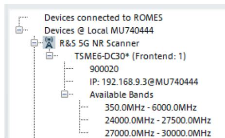
Figure 33: TSME30DC downconverter is automatically recognized as a front-end frequency extension in ROMES4.
