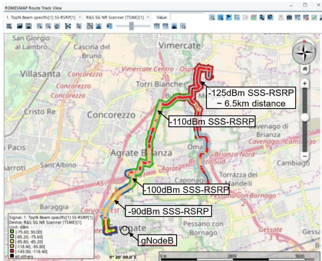
Figure 24: Drive test at 3.7 GHz in a suburban environment.
