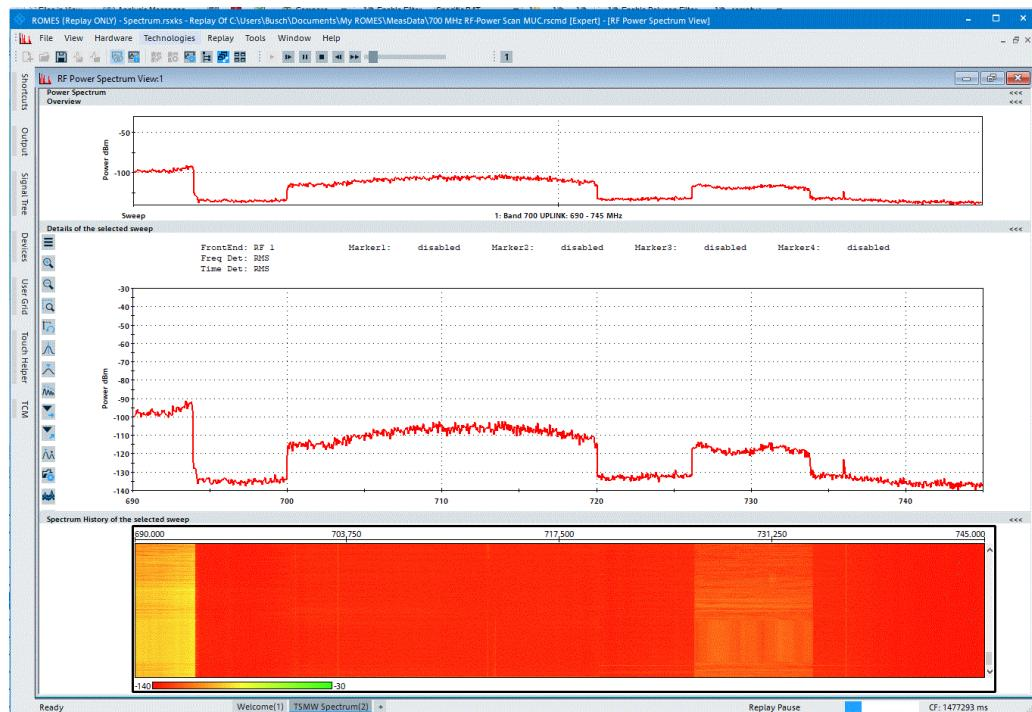
**Figure 39: Performing a spectrum scan for spectrum clearance with a R&S®TSMx network scanner and R&S®ROMES4**
