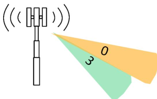
**Figure 59 SSB index 0 and 3 elevation**
