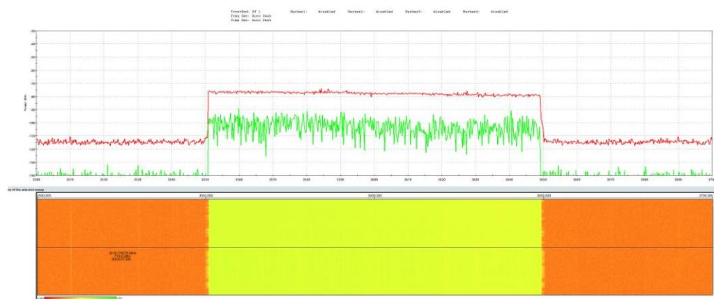
**Figure 44: Spectrum scan of a 5G NR carrier with four SSBs and UE specific signals (data traffic on air distributed over the whole 100 MHz 5G NR carrier)**
