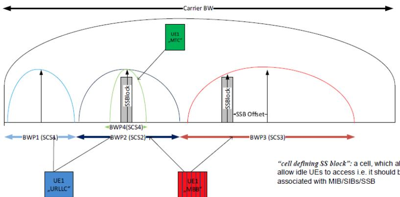
**Figure 4: 5G NR component carrier divided in bandwidth parts with own synchronization blocks**
