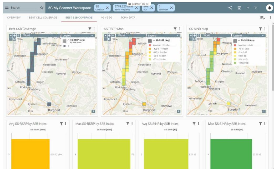
**Figure 53 5G Scanner Best SSB Coverage for PCI 487 and SSB index 3**
