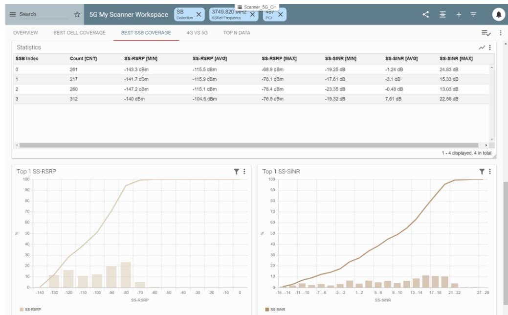
Figure 52 5G Scanner Best SSB Coverage for PCI 487, part 2
