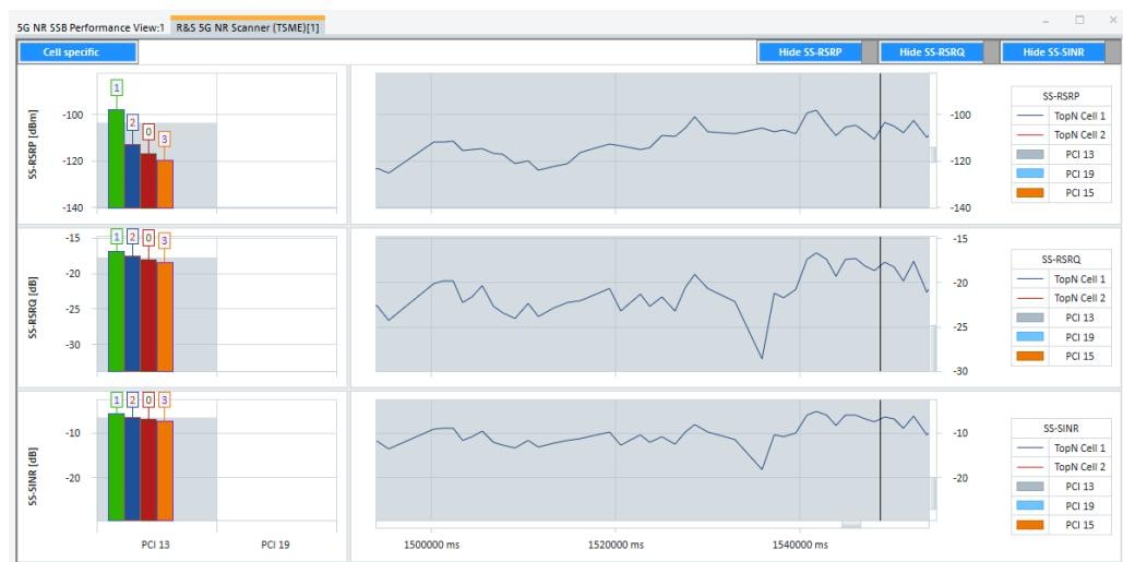
Figure 28: 5G NR Scanner SSB Performance View visualizing values from a Cell specific Top N Pool, with detailed RF results from PCI 13.
