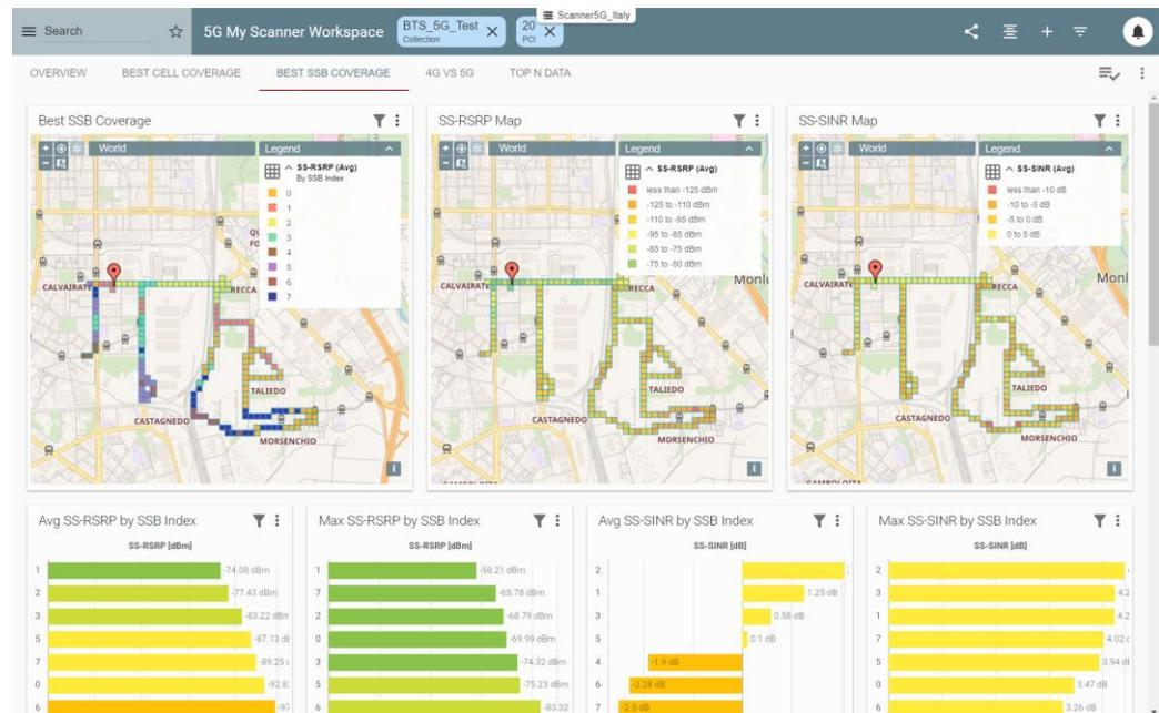
**Figure 54 5G Scanner Best SSB Coverage for PCI 20 having 8 different SSB indices**
