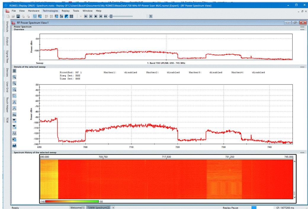
Figure 39: Performing a spectrum scan for spectrum clearance with a R&S@TSMx network scanner and R&S@ROMES4
