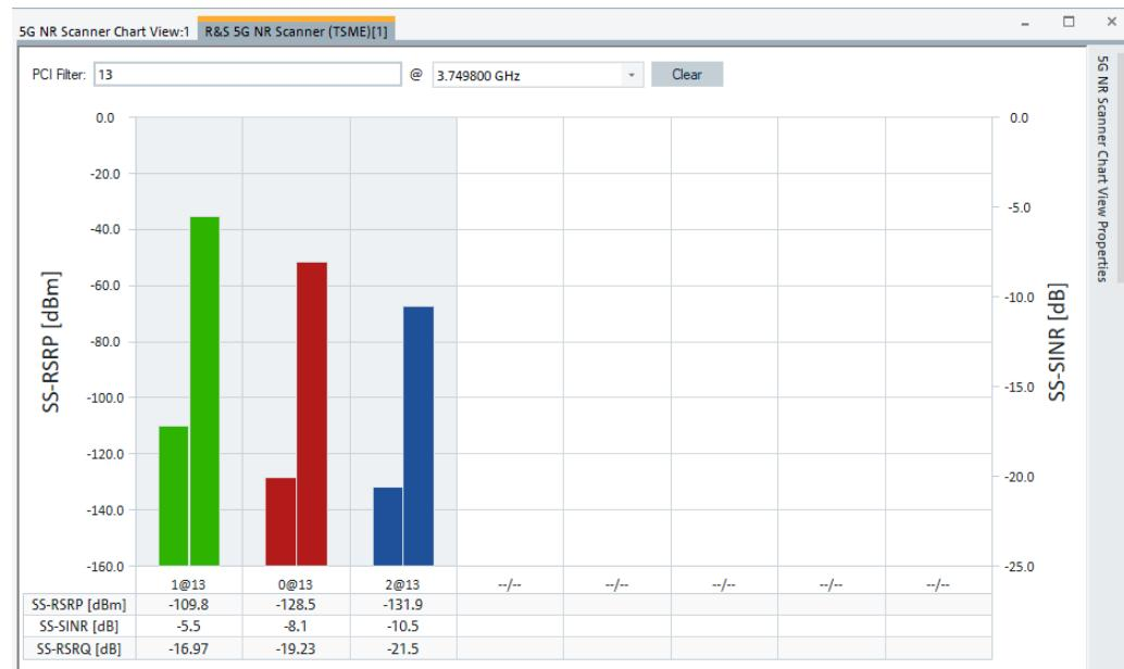
Figure 29: 5G NR Scanner Chart View filtered by PCI 13.
