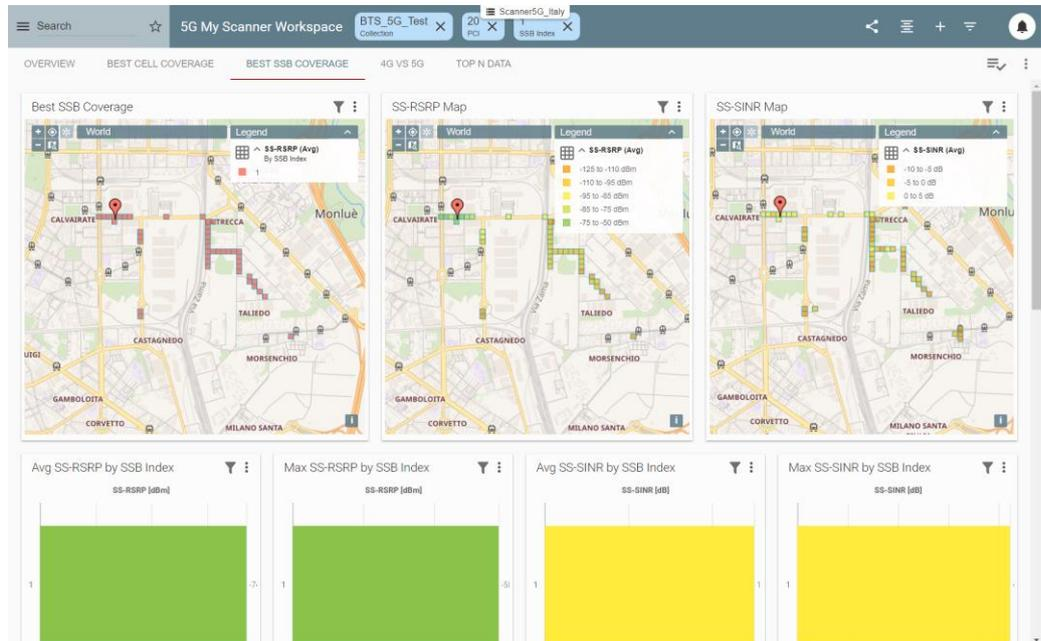
Figure 56 5G Scanner Best SSB Coverage for PCI 20 and SSB index 1
