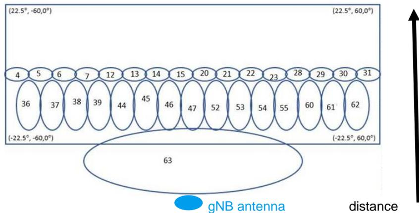
Figure 37: Beam pattern of a configuration with 32 SSBs / beams (projection on geographical area).
