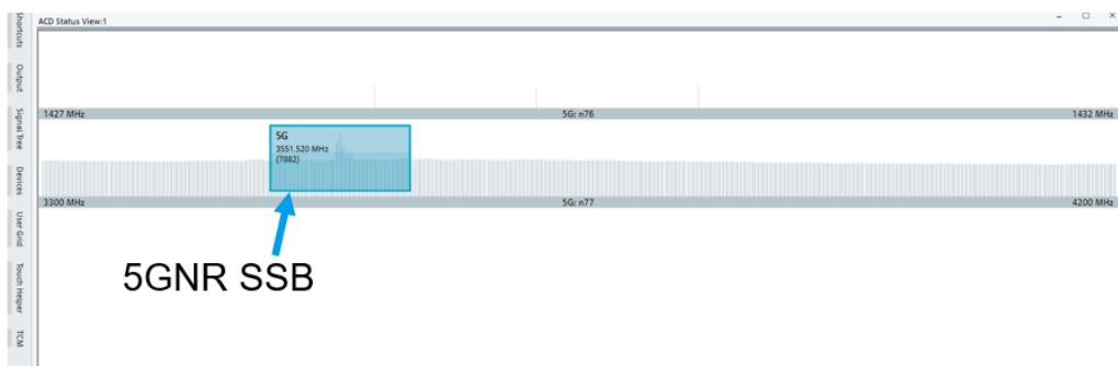
Figure 11: 5G NR ACD result in the ROMES4 ACD view
