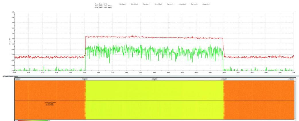
Figure 44: Spectrum scan of a 5G NR carrier with four SSBs and UE specific signals (data traffic on air distributed over the whole 100 MHz 5G NR carrier)
