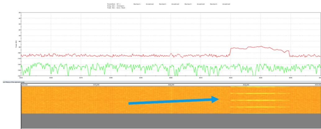
Figure 42: Spectrum scan of a SSB with small FFT size.
