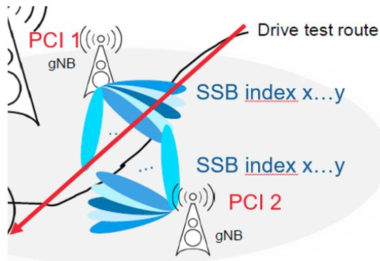
**Figure 9: Drive test crossing several SSBs and PCIs**
