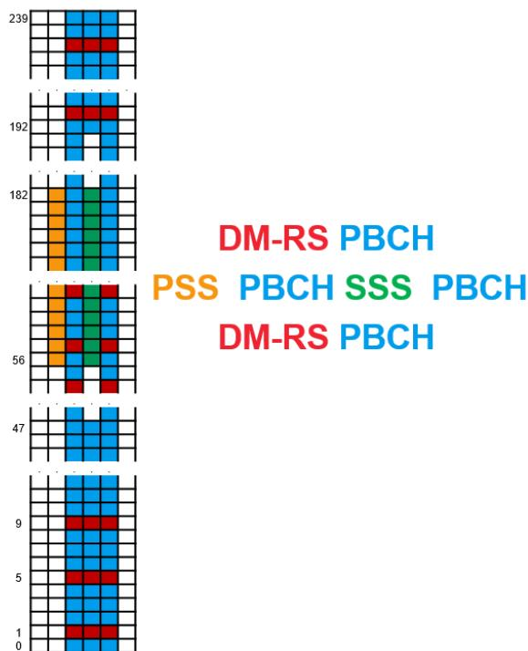
Figure 6: 5G NR synchronization block with increased zoom factor
