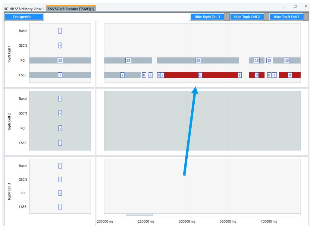
Figure 26: 5G NR scanner SSB History view indicating a change of the SSB index (same PCI)
