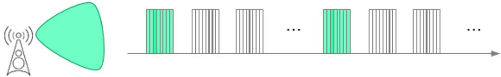
Figure 18: Multiple SSBs (green) transmit the same beam.
