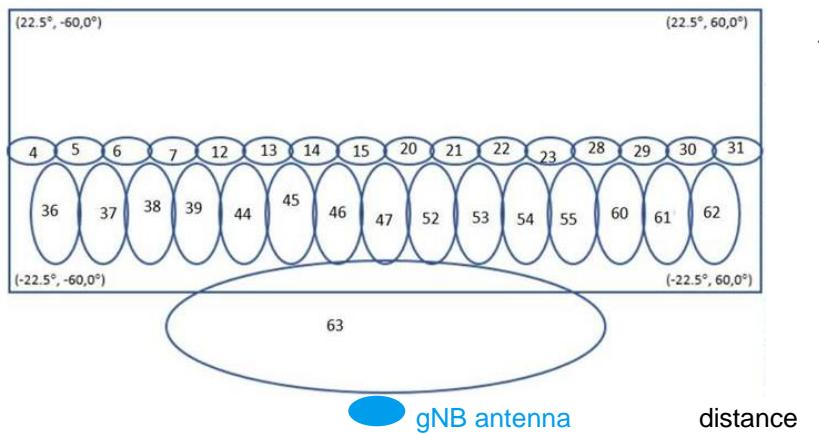
Figure 37: Beam pattern of a configuration with 32 SSBs / beams (projection on geographical area).
