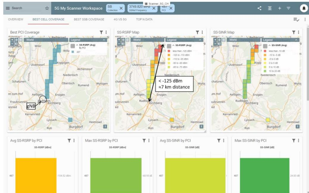
**Figure 50 5G Scanner PCI 487 coverage analysis**
