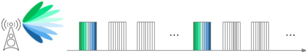
Figure 19: Individual SSBs (blue, grey, green) transmitted on multiple physical beams
