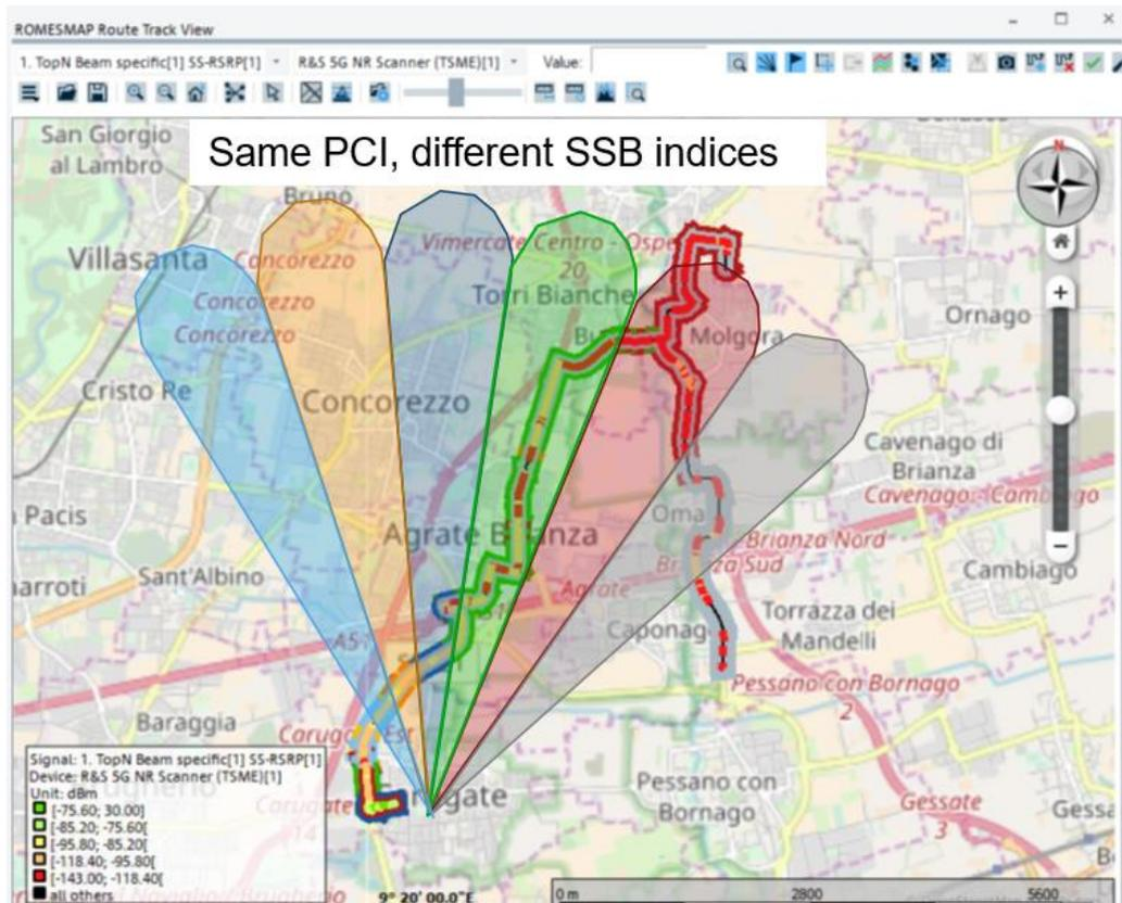
Figure 25: Mapping the potential beam coverage on the SSB index results.
