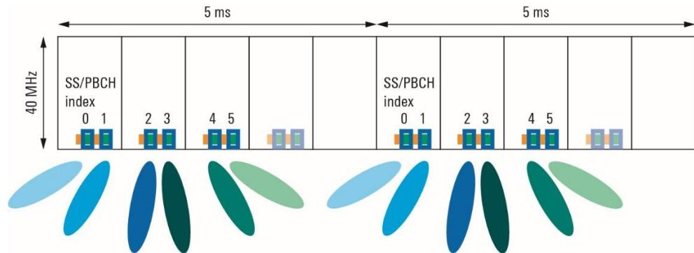
**Figure 8: Example of SSB transmissions**
