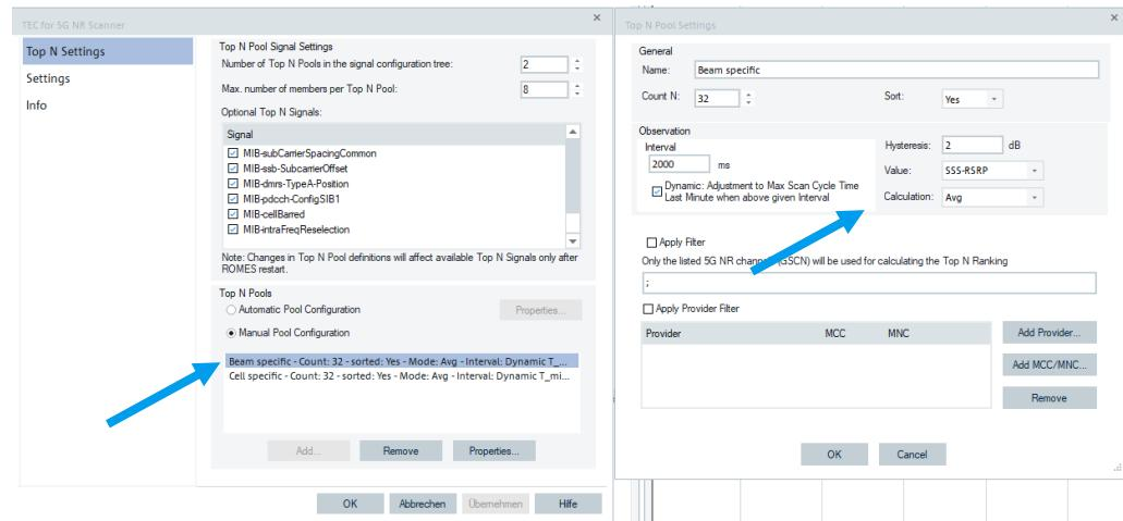
Figure 14: Top N Settings in ROMES4 for a Beam / SSB specific Top N Pool
