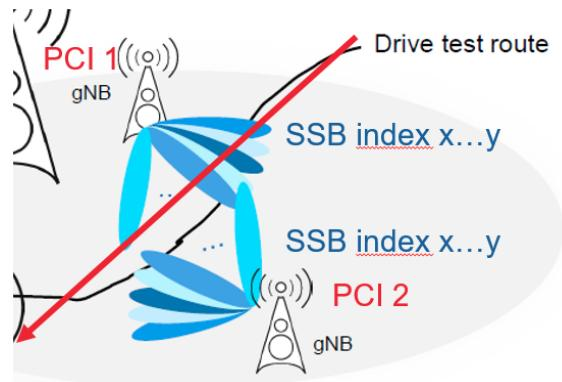
**Figure 9: Drive test crossing several SSBs and PCIs**
