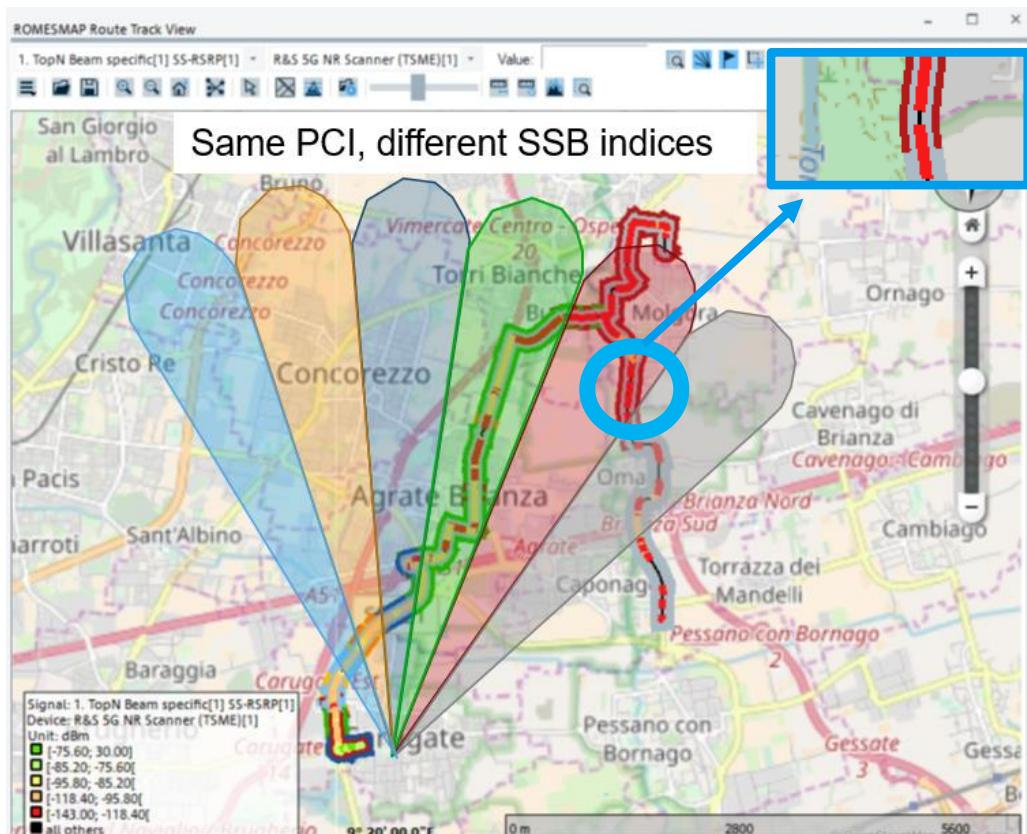
Figure 27: Change of SSB index on the map (highlighted with blue color)
