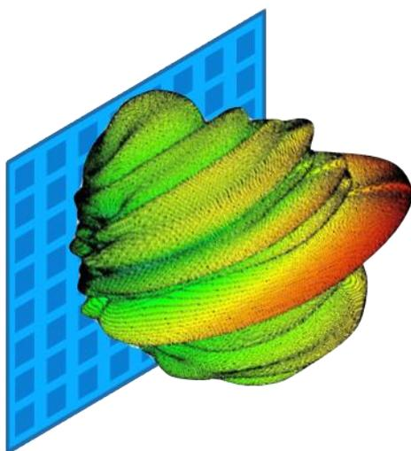
**Figure 2: Beamforming using an antenna array with phase shifting between antenna elements**
