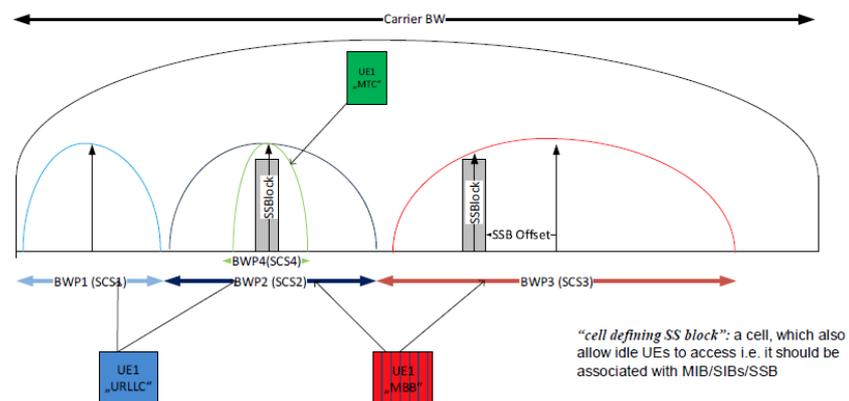
**Figure 4: 5G NR component carrier divided in bandwidth parts with own synchronization blocks**
