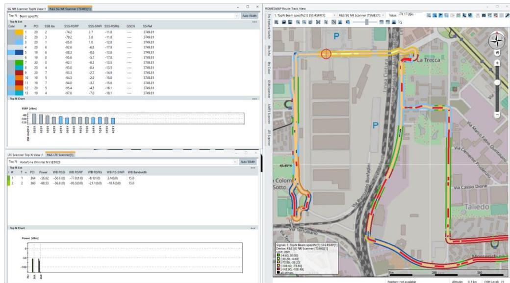
Figure 38: ROMES4 worksheet with the map, 5G NR and LTE scanner Top N View.
