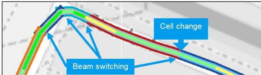
Figure 23 ROMES4 Map example of Beam specific Top N plot
