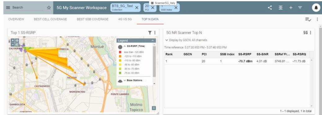
Figure 57 5G Scanner Top N Data with PCI 20 and SSB index 1 cell sector coverage lines
