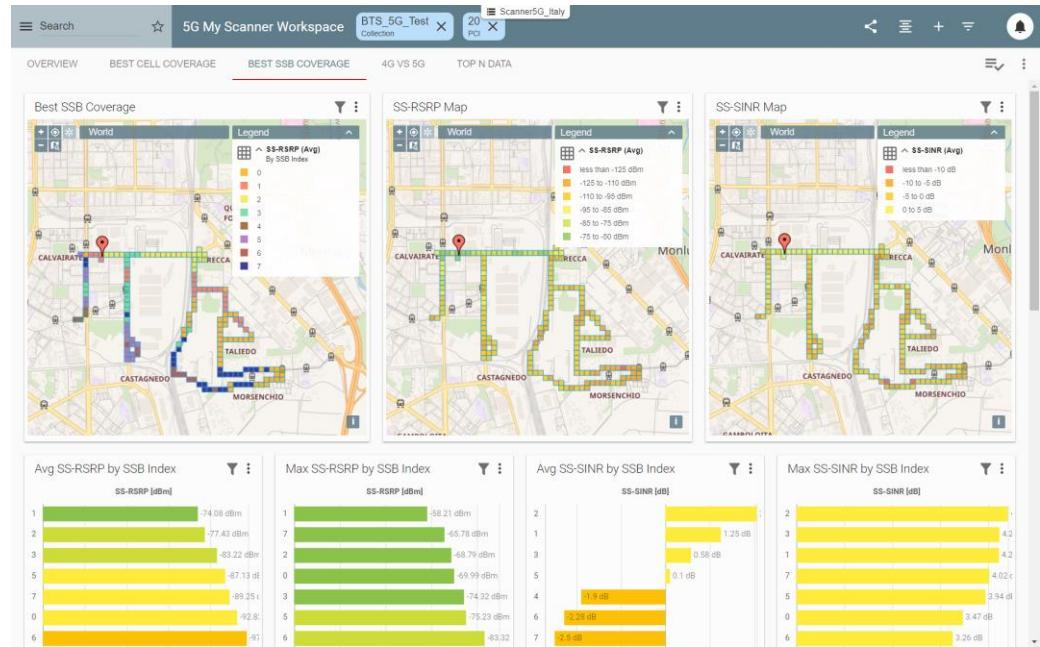
Figure 54 5G Scanner Best SSB Coverage for PCI 20 having 8 different SSB indices
