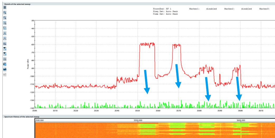
Figure 43: Spectrum scan of four SSBs with a higher FFT size.
