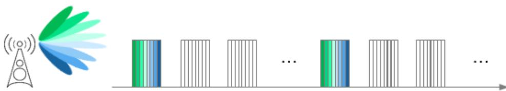
Figure 19: Individual SSBs (blue, grey, green) transmitted on multiple physical beams
