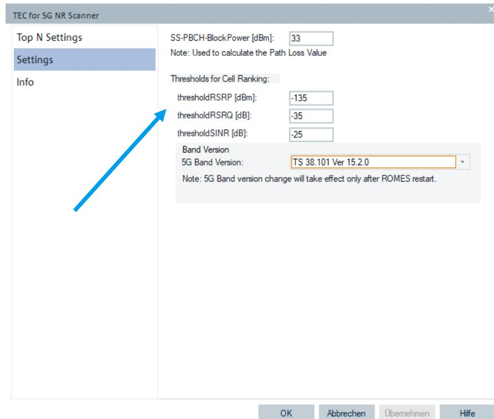
Figure 17: Setting thresholds for PCI / cell based Top N Pools.
