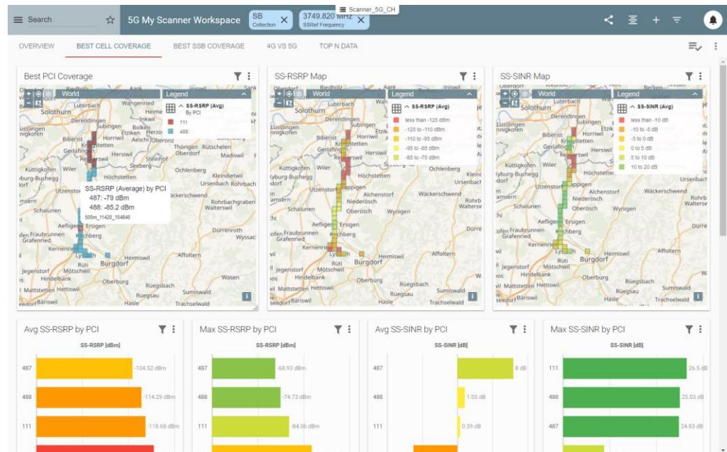
Figure 49 5G Scanner Best cell coverage analysis
