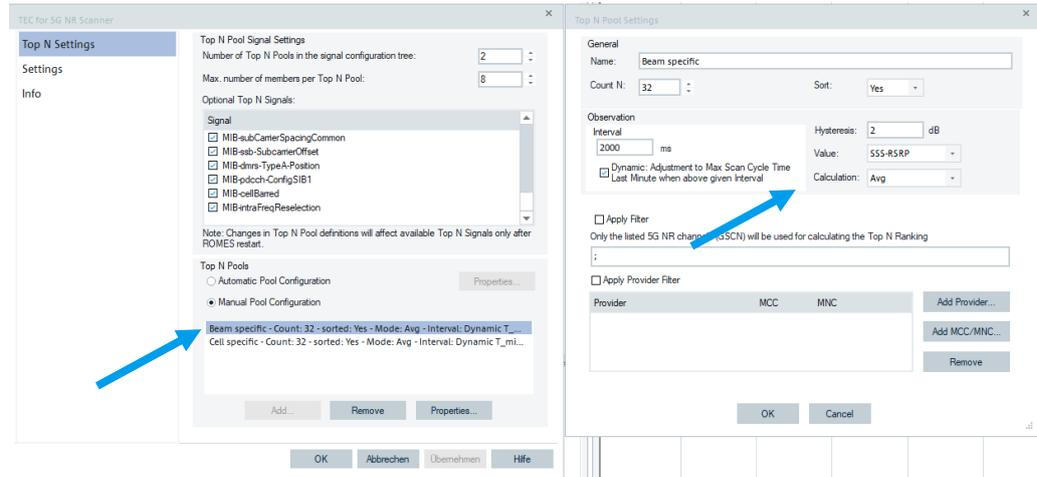
Figure 14: Top N Settings in ROMES4 for a Beam / SSB specific Top N Pool
