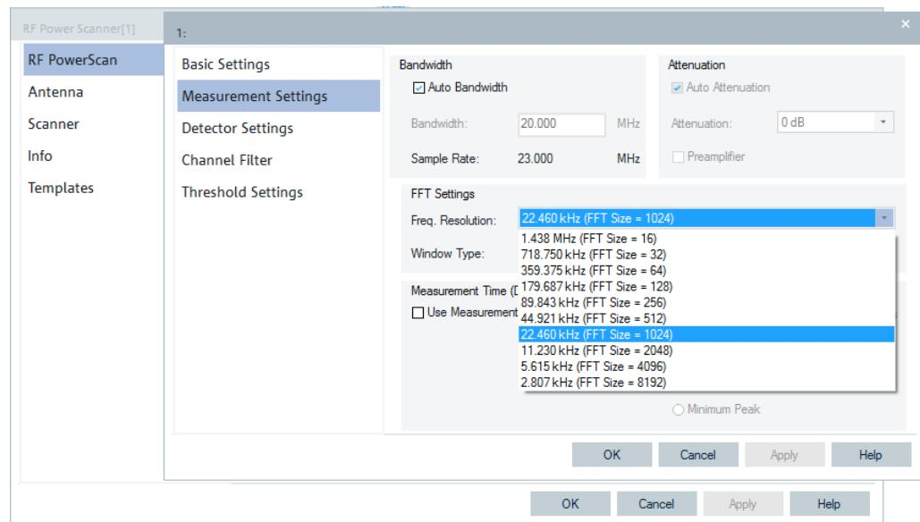
**Figure 41:** RF power scan FFT size / frequency resolution settings to change the resolution in time and frequency.
