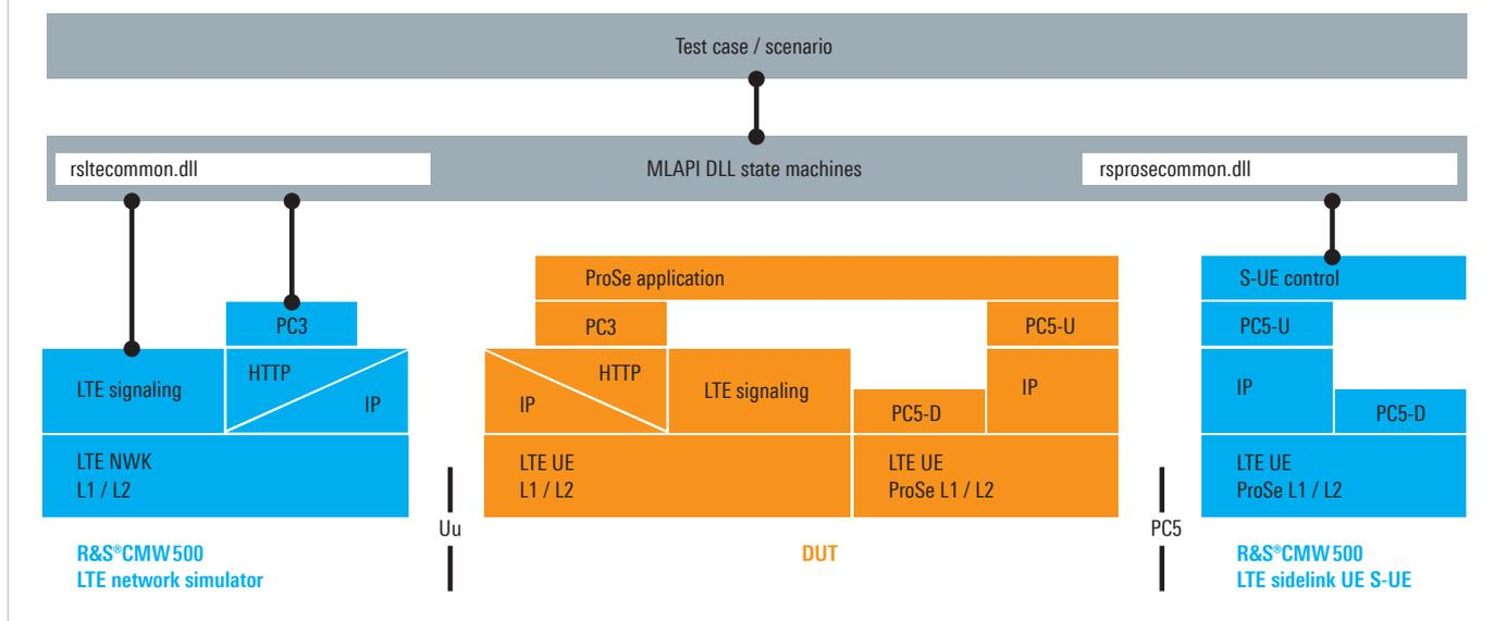
Fig. 3: Test architecture for ProSe tests, consisting of the R&S<sup>®</sup>CMW500 (blue) and the mobile device (DUT).
