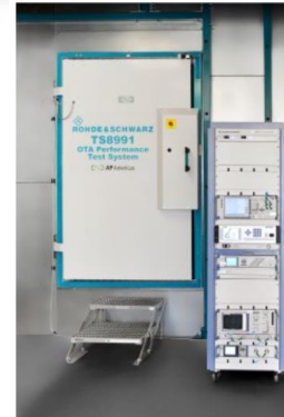
WPTC shielded room • PCV/PCO
