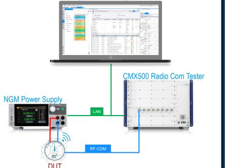
The R&S®CMX500 Battery Life Testing solution offers seamless power consumption measurements in parallel to:
