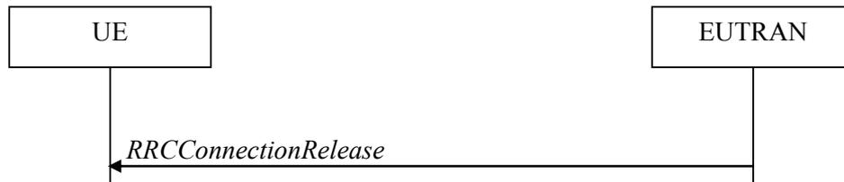
図 2: RRC connection release procedure [8]
