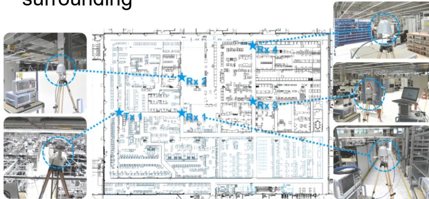
Power delay profile measurements in the factory
