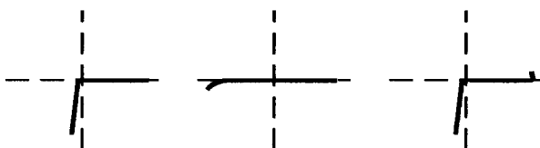
Typ: Normale Diode Hochspann.-Diode Z-Diode 6,8V Pole: Kathode-Anode Kathode-Anode Kathode-Anode Anschlüsse: (CT - Masse) (CT - Masse) (CT - Masse)
