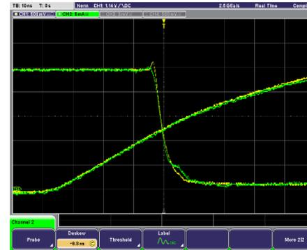
Current and voltage pulse aligned
