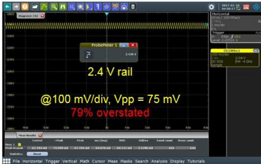
Using built-in probe offset
