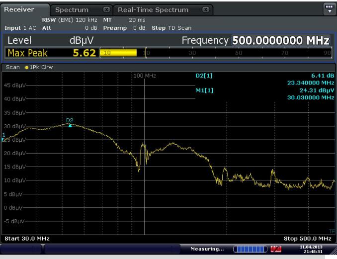
TV Set near power connector; transducer H-nearfield probe
