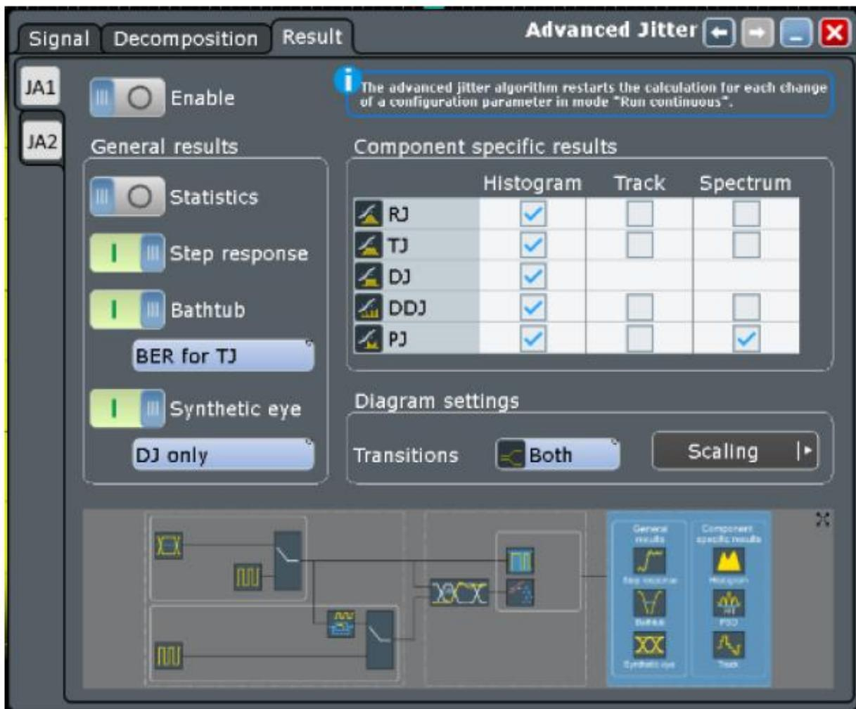
Figure 10: Setup step 3 - Select the results displays
