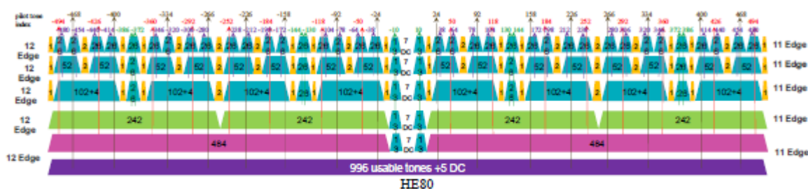
Fig. 4-6: 80 MHz Resource Unit and Tone Allocations [7]
