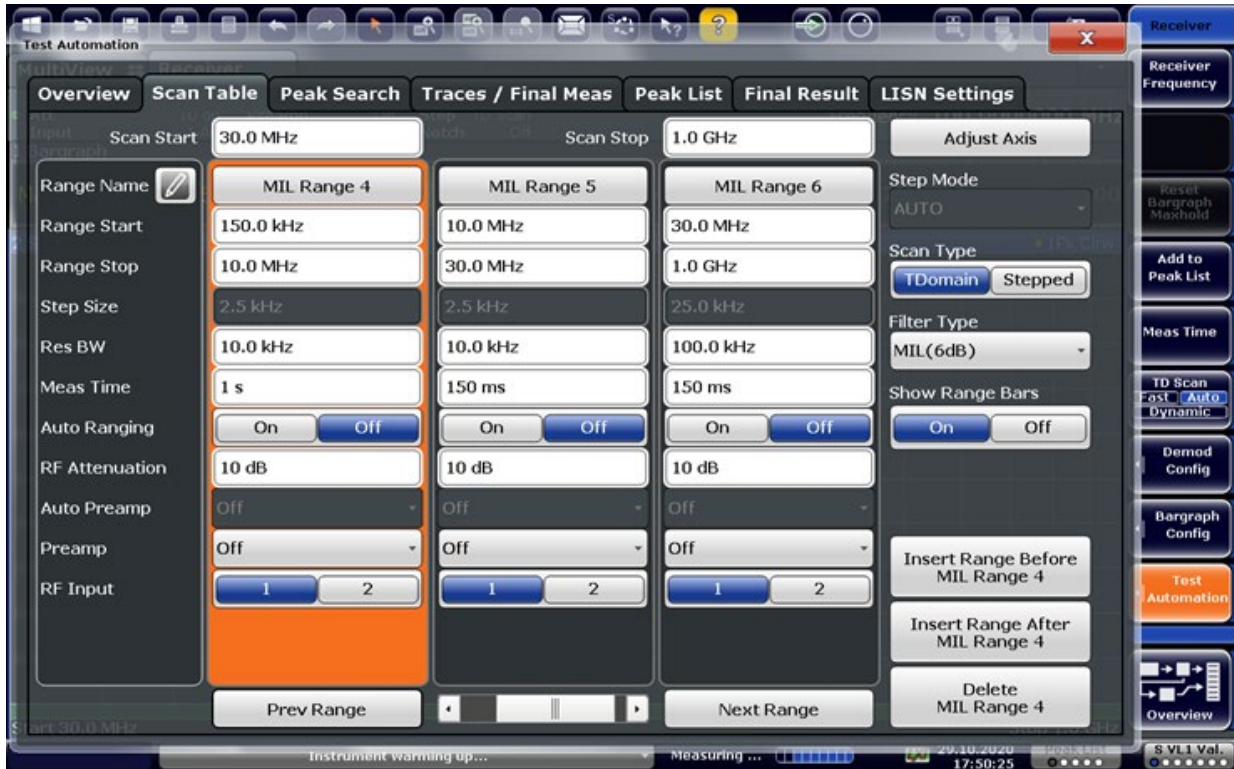
Figure 7. Modern EMI receivers simplify setup and reduce access to compliant parameters. In this example, measurement time is the only user-accessible variable.
