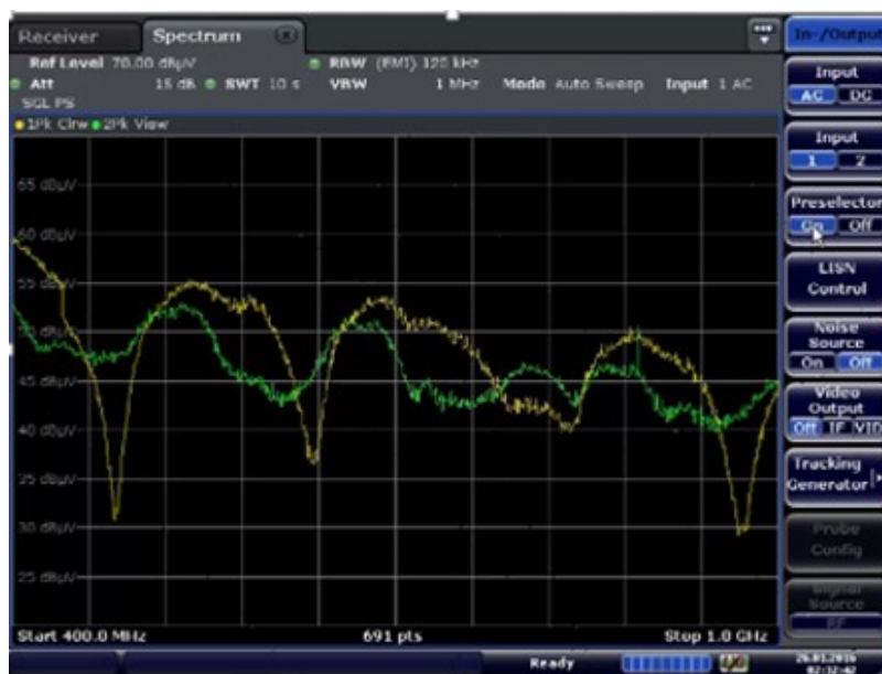
Figure 4. Without preselection (green trace), incoming signals may overload the receiver front-end. Preselection (yellow trace) helps prevent bad data and ensure valid measurement results.
