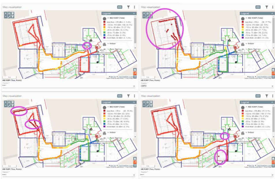
Figure 4 The maps above show the LTE coverage RSRP on CBRS and across three major carriers. Anticipated gaps in coverage are circled on the map.
