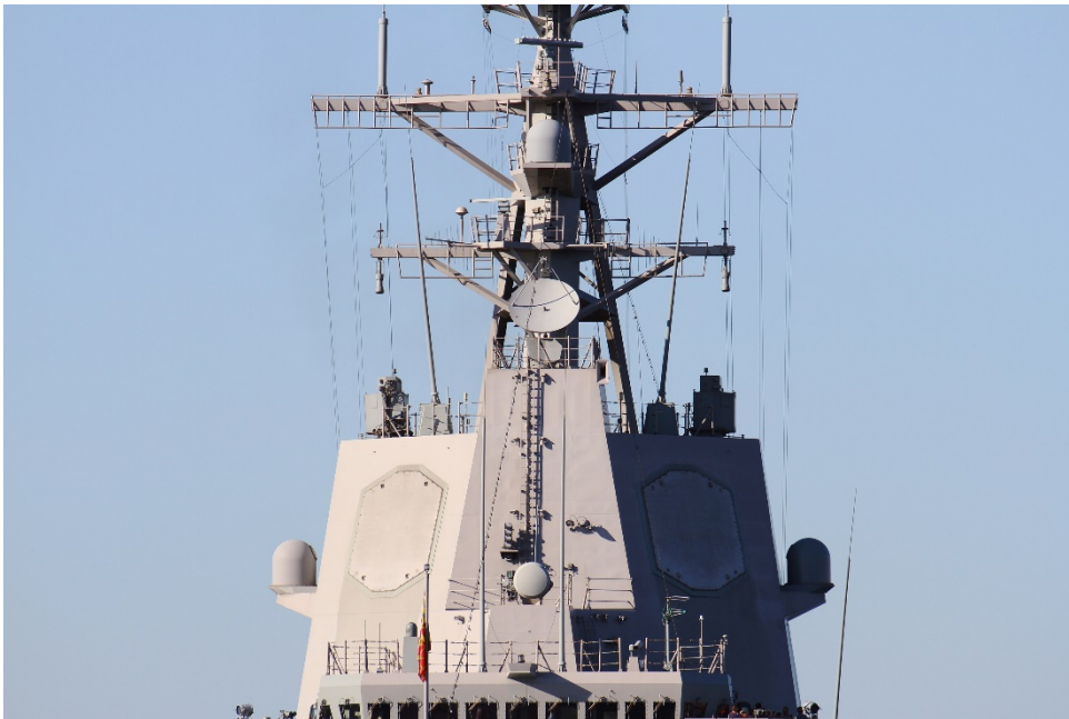
Figure 10: Navy Ship Mast Antenna Example
